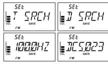
6. When the radio detects the correct tone or code, it will halt on that tone/code, and audio will be allowed to pass. Press the [BAND] key to lock in that tone/code, then press and hold the [TXPO] key for one second to exit to normal operation.
