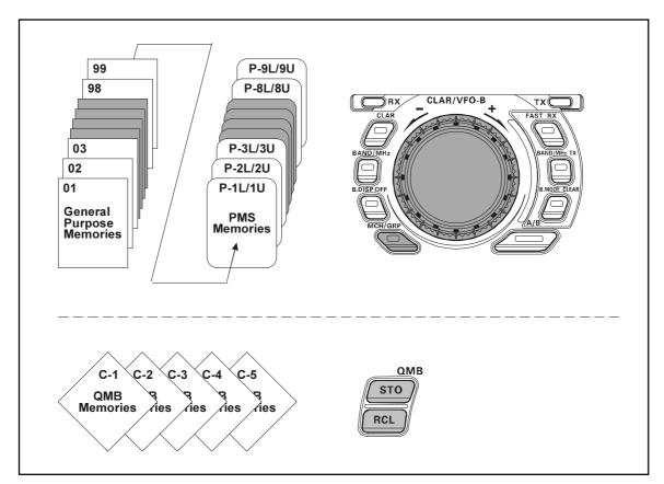
The Quick Memory Bank is comprised of five memories (labeled "C1" ~ "C5") independent from the regular and PMS memories. These can quickly store operating parameters for later recall.
