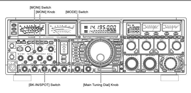
Before starting, connect your key line to the front and/or rear panel [**KEY**] jack, and be sure the [**KEYER**] switch on the left side of the front panel is turned off for now.
