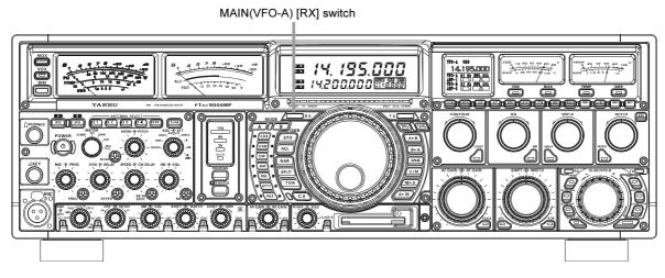
Press the Main (VFO-A) band's [RX] LED/switch.
