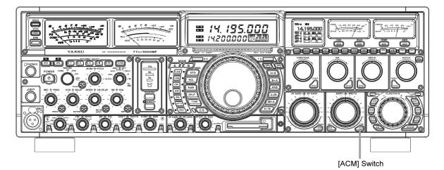
To activate the Adjacent Channel Monitor, press the **[ACM**] switch. The LED imbedded in the switch will glow Red.
