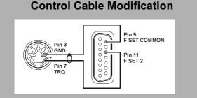
Please cut off the RCA connector on one end of the CONTROL Cable supplied with the **VL-1000**, and install a 7-pin DIN connector in its place, according to the illustration.
