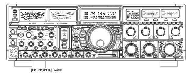
Rotation of the front panel's **[CW PITCH]** control will allow adjustment of the center frequency of the receiver passband, as well as the pitch of your offset CW carrier, to the tone you prefer. The tone may be varied between 300 Hz and 1050 Hz, in 50 Hz steps.
