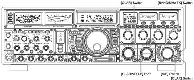
Press the [CLAR] switch. The Red LED imbedded in the switch will light up, and "CLAR" will appear in
