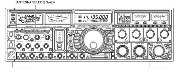
Selection of the desired TX/RX antenna is accomplished by pressing the appropriate  $[1] \sim [4]$  Antenna Selection switch on the front panel.
