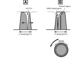
To switch the IF Notch filter off, press the Sub (VFO-B) band's **[NTCH]** switch once more. The LED imbedded in the switch will turn off, confirming that the IF Notch filter is no longer operating.
