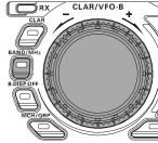
When tuning in 1 MHz steps, clockwise rotation of the [**CLAR/VFO-B**] knob will increase the frequency, while counter-clockwise rotation will cecrease the frequency.
