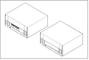
Linear Amplifier / AC Power Supply VL-1000 / VP-1000
