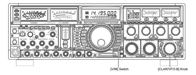
To operate on the 60-meter band channels, press the [V/M] key, if necessary, to enter the Memory mode, then rotate [CLAR/VFO-B] knob to select the desired channel from the above selections.
