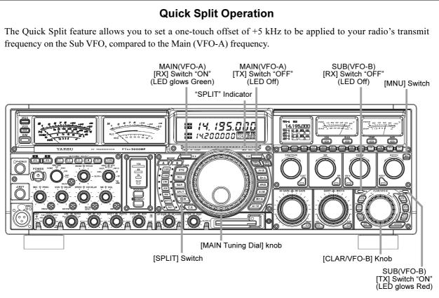
1. Start with regular transceiver operation on the Main (VFO-A) band.
