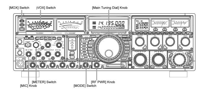
The operating mode is selected using the [MODE] switches to the left of the [MAIN Tuning Dial] knob, and the VFO (A or B) to which the selection is applied is selected by pressing the [A] or [B] switch above the Mode keys. Press the [A] or [B] key to select the desired VFO, then press the [LSB] or [USB] key to select one of the SSB modes. For AM operation, press the [AM] key.
