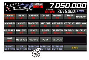
3. To u ch [DISPLAY] → [SCREEN SAVER] or rotate the [FUNC] knob to select an item and press the [FUNC] knob.
