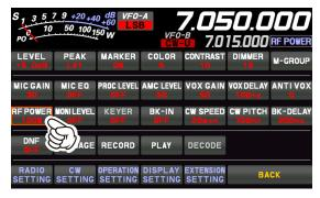
Rotate the [FUNC] knob to adjust the RF power.
