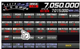
Rotate the [FUNC] knob to adjust the Monitor level.
