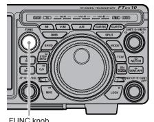
The last function used is retained in the [FUNC] knob so it can be easily set by operating the [FUNC] knob. Normally, it is suggested to utilize the [FUNC] knob as the [LEVEL] knob for the spectrum scope.
