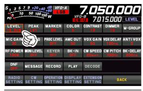
· On the 3DSS screen, weak signals may be more easily observed by adjusting the LEVEL so that the noise level can be seen only a little, so always adjust the LEVEL and use it at the optimum position.
