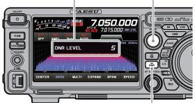
Press and hold the [DNR] key to display the DNR level.
