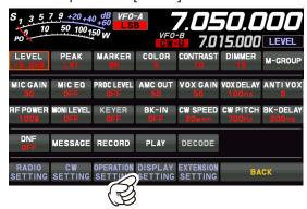
To u c h [DISPLAY] → [LED DIMMER] or rotate the [FUNC] knob to select an item and press the [FUNC] knob.
