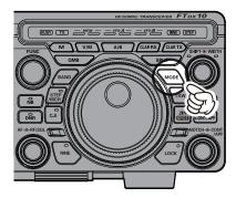
2. The operation MODE selection screen appears on the display, then touch [PRESET], or rotate the MPVD ring to select [PRESET].
