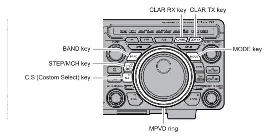
BAND: Press the [BAND] key and then rotate the MPVD ring to switch the operating frequency band.
