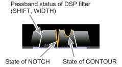
The current roofing filter bandwidth is displayed as a blue line below the filter function display.
