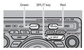
During Split operation, the VFO-A register will be used for reception, while the VFO-B register will be used for transmission. If you press the [SPLIT] key once more, Split operation will be cancelled.
