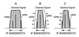
For best interference reduction, the WIDTH and SHIFT features are the primary tools you should use. After narrowing the bandwidth (WIDTH) and/or adjusting the center of the passband (SHIFT), the Contour control may then yield additional signal-enhancement benefits on the net residual bandwidth. Even more, the IF NOTCH Filter (described later) may also be used, in conjunction with these filter systems, to significant advantage.
