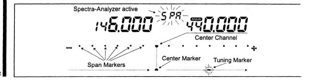
It is important to realize that the total spectrum you can view depends on the configuration of three (3) following settings:
