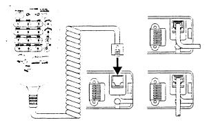
Important! Ensure the power is first switched off before removing the front sub-panel. The transceiver will turn off automatically after two seconds if the front panel is removed with power applied.
