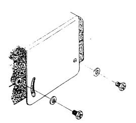
☐ Position the transceiver in the bracket so that the holes in the side are aligned with those in the bracket, and bolt the transceiver into place using the supplied short screws and flat washers. The MH-39 hanger may be installed wherever convenient.
