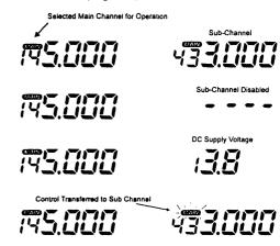
There are two ways to select or toggle the main channel of operation. You can momentarily press either ..., or the DIAL knob to toggle the desired channel. Remember to only press these for less than ½ sec, as holding them longer will turn the transceiver off.
