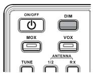
You may also customize the amount of brightness reduction engaged by the pressing of the [DIM] button, and may use different brightness levels for different front panel areas. Menu item "008 diSP DIM MTR" adjusts the brightness level of the analog meter; while menu item "009 diSP DIM VFD" sets the brightness levels of the frequency display (these settings are effective only when the [DIM] button is pressed).
