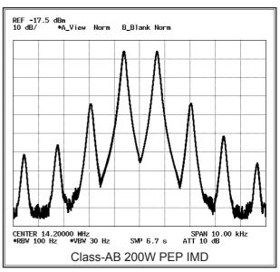
☐ The High-Power 200-Watt Final Amplifier Stage of the **FT-2000D** utilizes a pair of ST Micro Electronics Corp. SD2931 MOSFET devices operating at 50 Volts. The push-pull configuration provides low distortion along with high power output. The 92 mm thermostatically-controlled cooling fan directs forced air across the heat sink, when triggered by a rise in heat sink temperature.
