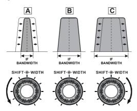
The default bandwidths\*, and total bandwidth adjustment range, will vary according to the operating mode:
