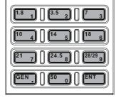
2. Press, in order, the digits of the operating frequency, using the [BAND] buttons (which have the frequency-entry digit or decimal point on the right side of the slash bar). In this example, enter
