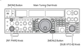
9. When you have completed all adjustments, press and hold in the [MENU] button for two seconds to save the new settings and exit to normal operation. If you only press the [MENU] button momentarily to exit, any changes you performed will not be stored.
