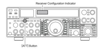
2. To restore full signal strength through the Attenuator circuit area, press the [ATT] button to restore the ATT display to the "OFF" position.
