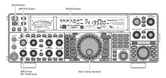
1. The operating mode is selected using the [MODE] buttons to the left of the Main Tuning Dial knob, and the VFO (A or B) to which the selection is applied is selected by the [A] or [B] button above the [MODE] buttons. Usually, the [A] button glows Red, signifying
