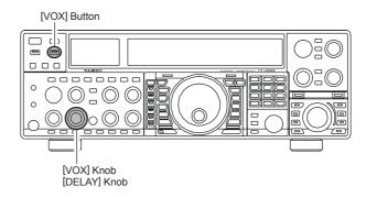
5. To exit from VOX operation, press the **[VOX]** button once more. We recommend doing this if you are going to leave your station, to prevent inadvertent activation of the VOX system by a ringing nearby telephone, speaker audio from a TV, etc.
