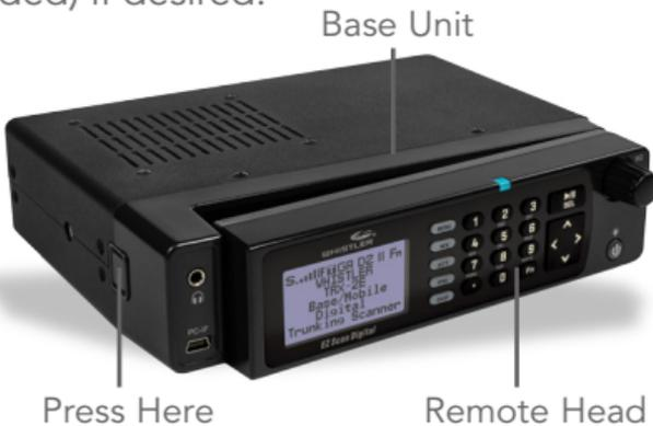
**WARNING:** Always install the remote head with care, keeping your fingers clear; the magnets are very powerful. Always keep the magnets well away from persons wearing electrical medical devices such as pacemakers, as the magnets may cause the devices to malfunction, endangering the wearer's life.
