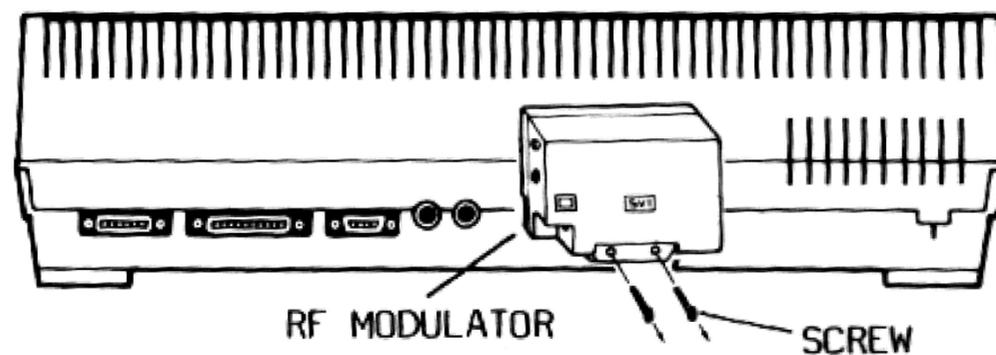
Fig. 2.5 Connecting an RF Modulator
