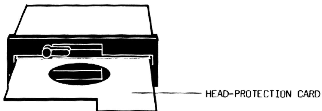
Fig. 2.2 Removing the Head-protection Card
