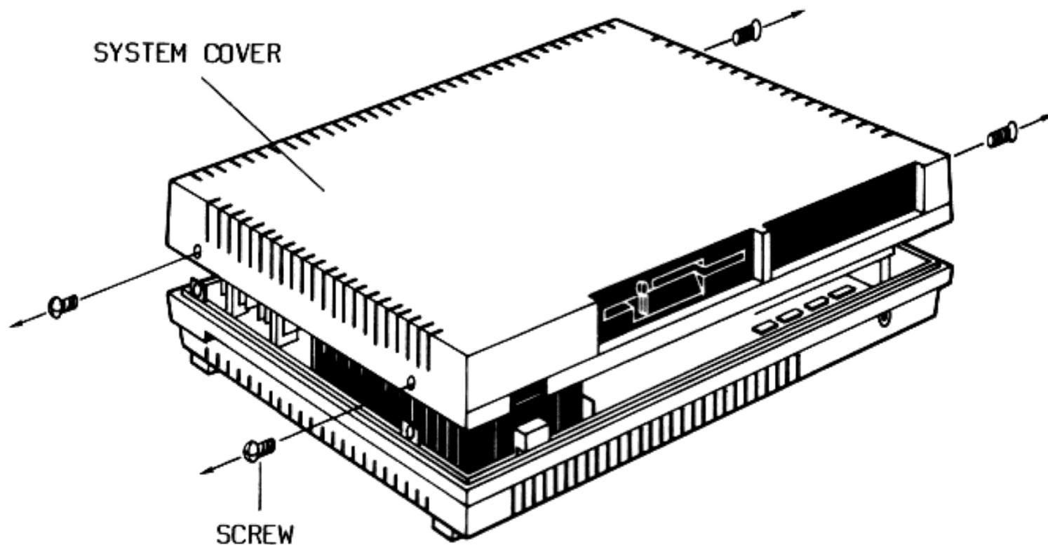
Fig. 2.6 Removing the Cover of the System Unit
