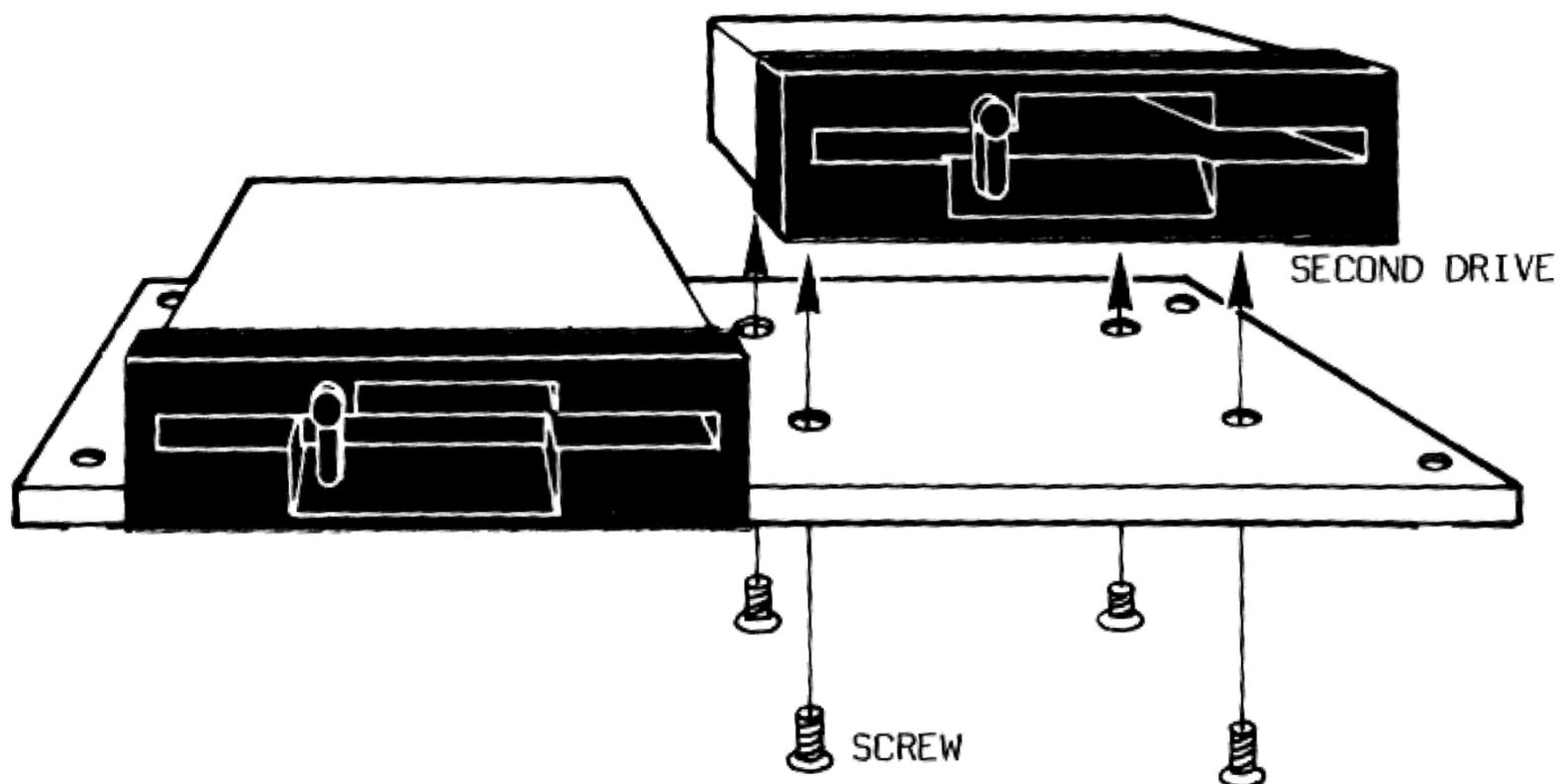
Fig. 2.9 Screwing the Second Drive onto the Mounting Plate
