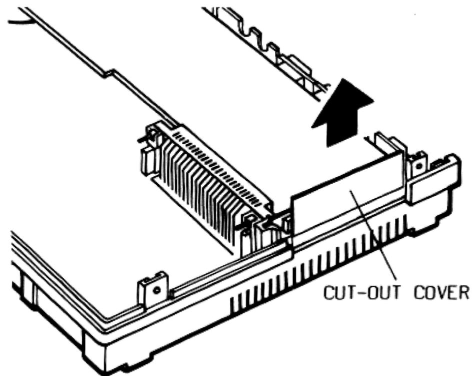
Fig. 2.14 Twisting off the Cut-out Cover
