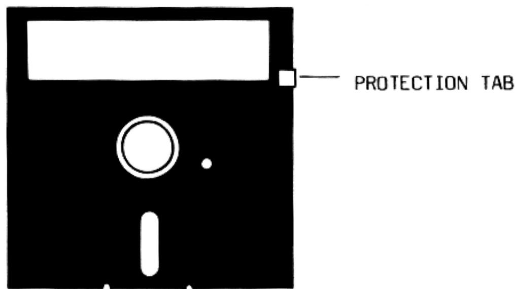
Fig. 1.4 Write-protecting a Disk
