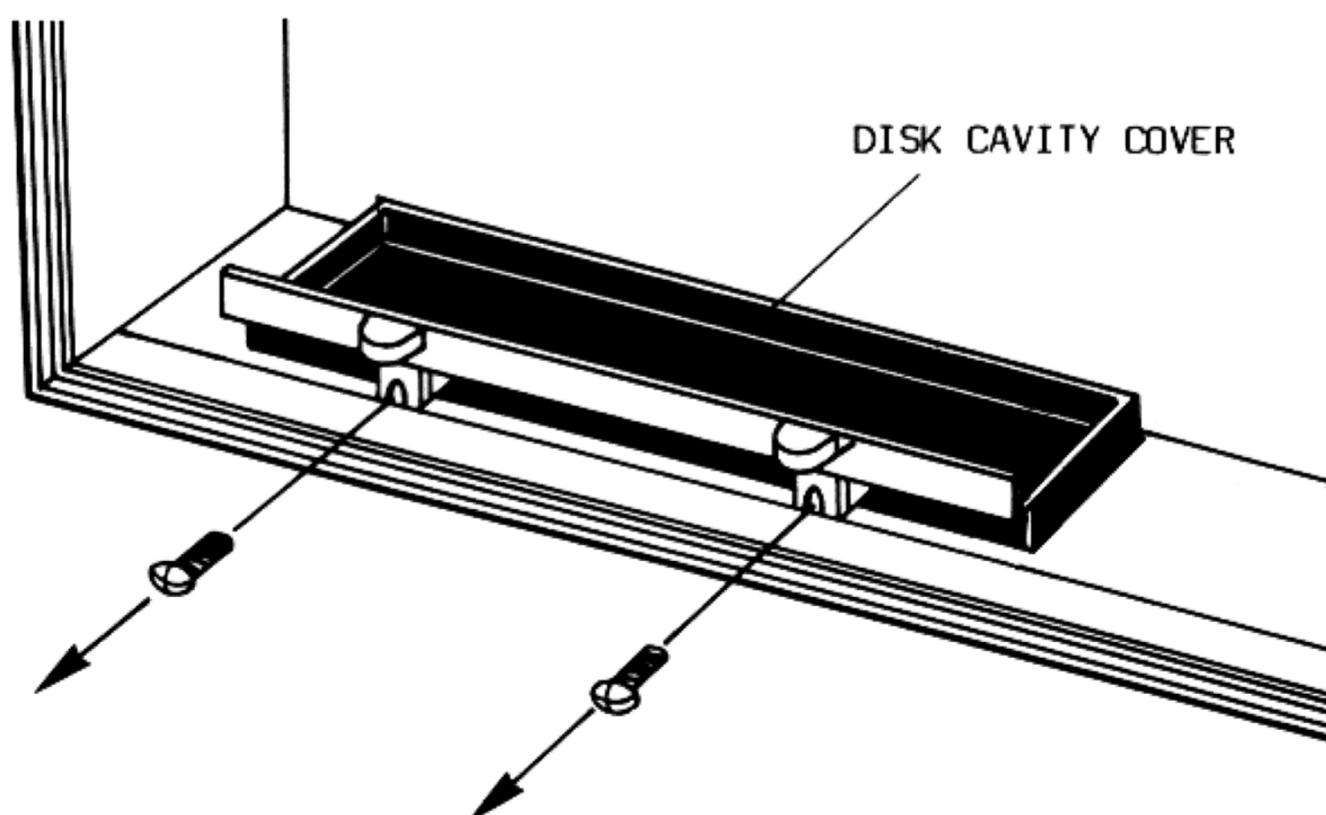
Fig. 2.7 Pushing out the Disk Drive Cover
