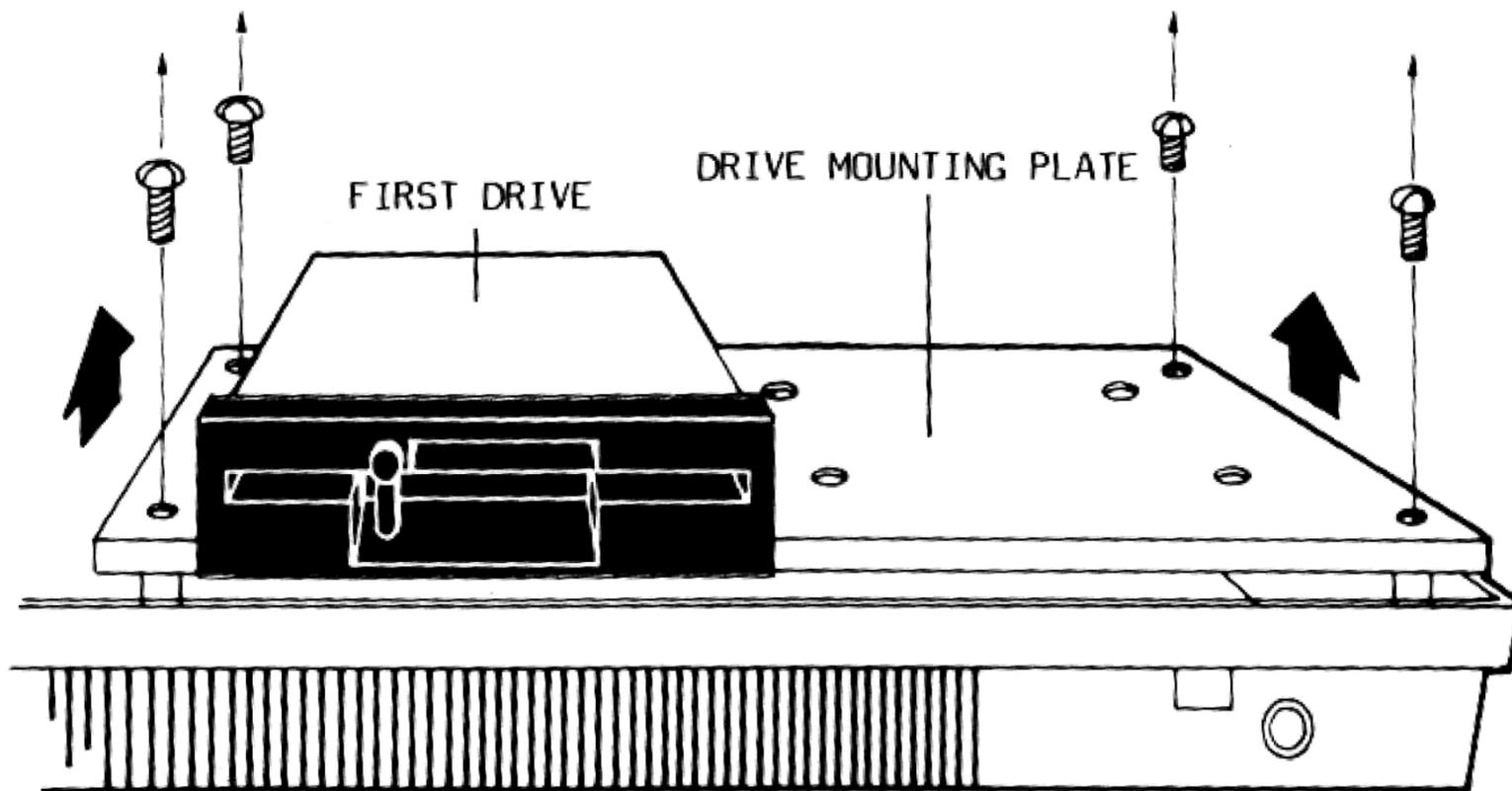
Fig. 2.8 Removing the Drive Mounting Plate
