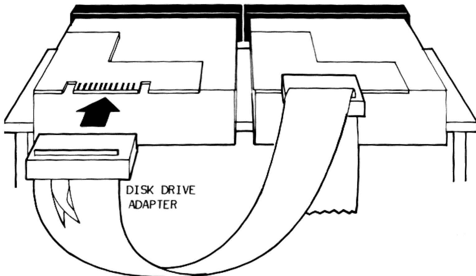
Fig. 2.11 Connecting the Disk Drive Adapter to the Second Drive
