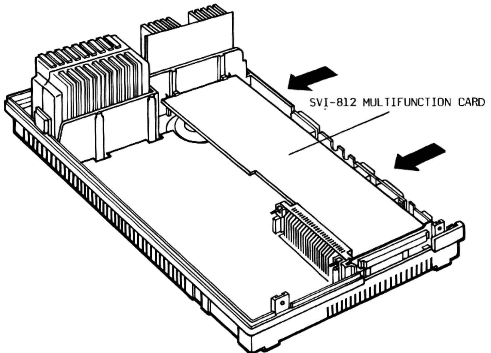
Fig. 2.12 Inserting the SVI-812 Multifunction Card
