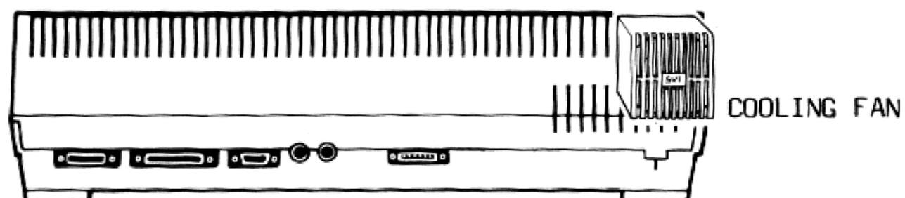
Fig. 2.18 Attaching the Fan to the Computer
