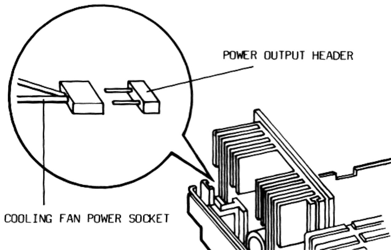
Fig. 2.17 Connecting the Power Supply
