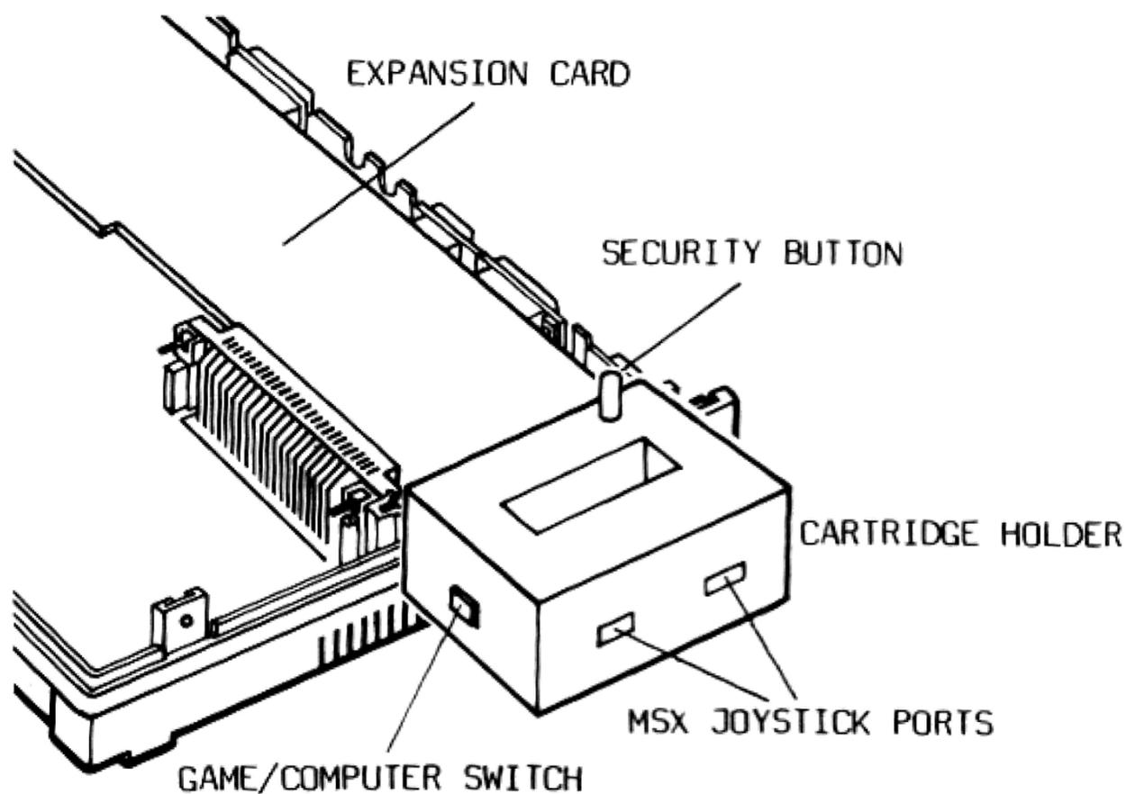
Fig. 2.15 Connecting the Cartridge Holder and Expansion Card
