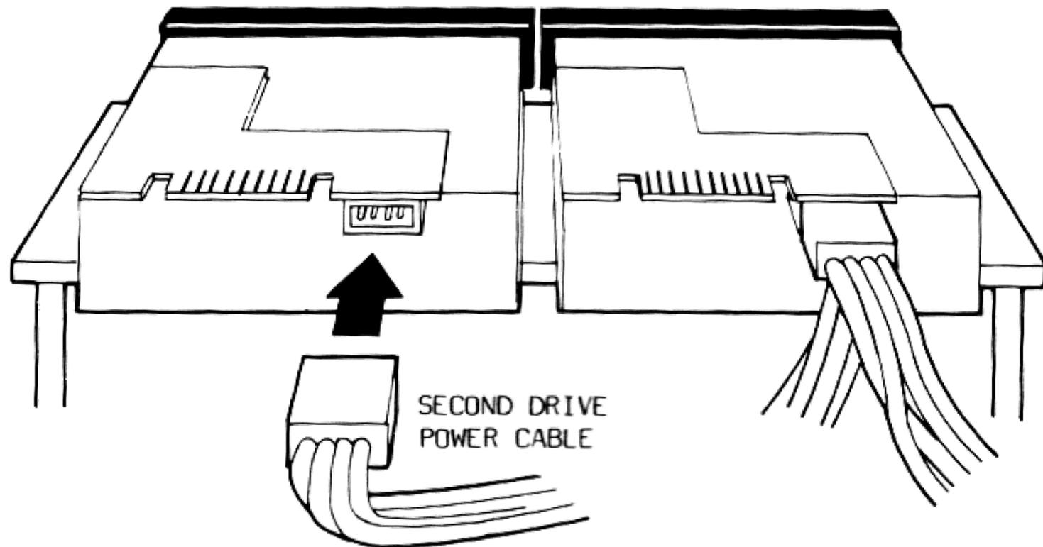
Fig. 2.10 Connecting the Power Cable to the Disk Drive
