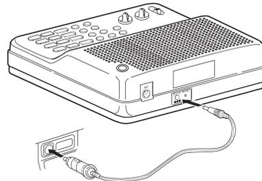
1. Connect the adaptaplug connector to the DC cord so the tip reads positive (+).
