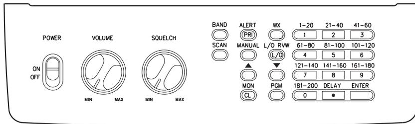
**POWER** — turns the scanner on and off.
