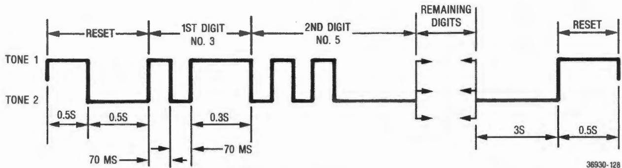
Figure 1-3. MTS Sequence Timing
