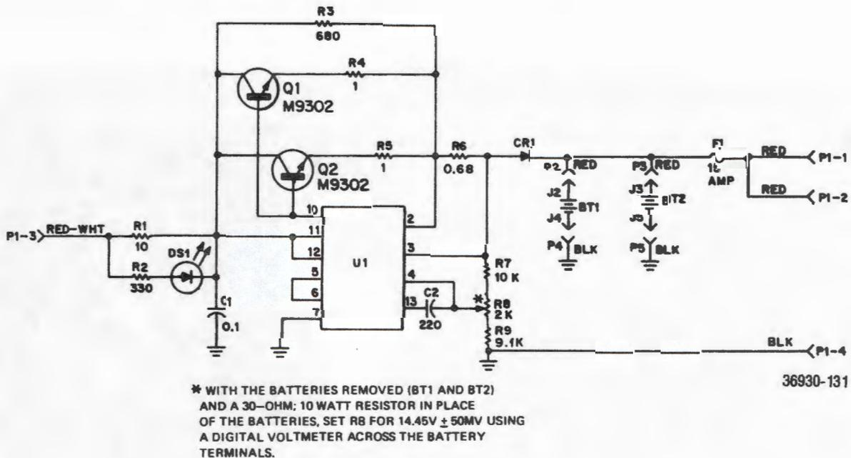
Figure 19-2. Battery Pack - Schematic
