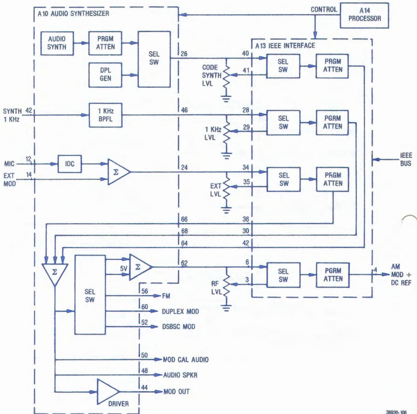
Figure 2-7. Code Synthesizer - Block Diagram
