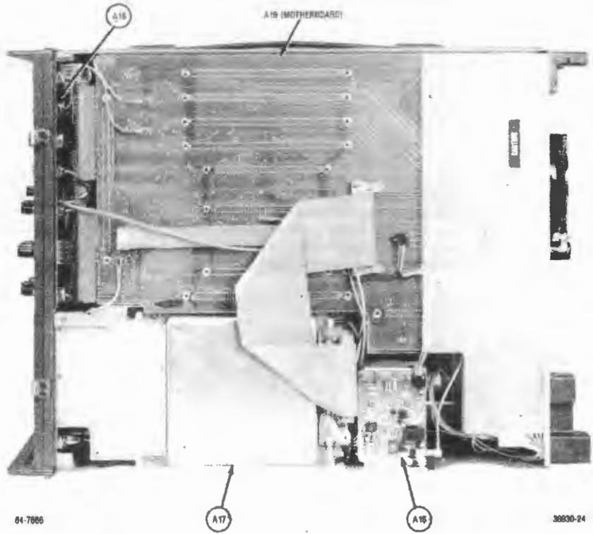
Figure 1-6. Communications System Analyzer — Bottom View, Cover Removed
