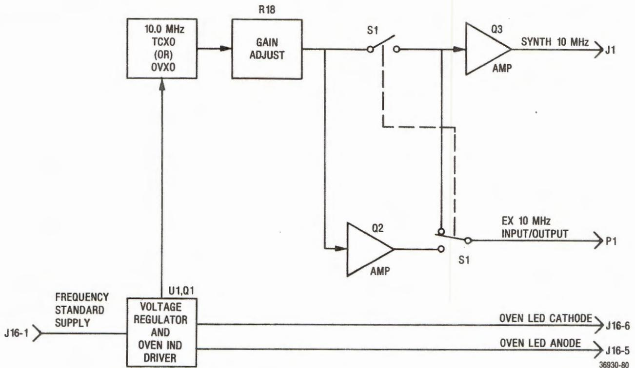
Figure 16-1. Frequency-Standard Interface Board (A16) — Block Diagram
