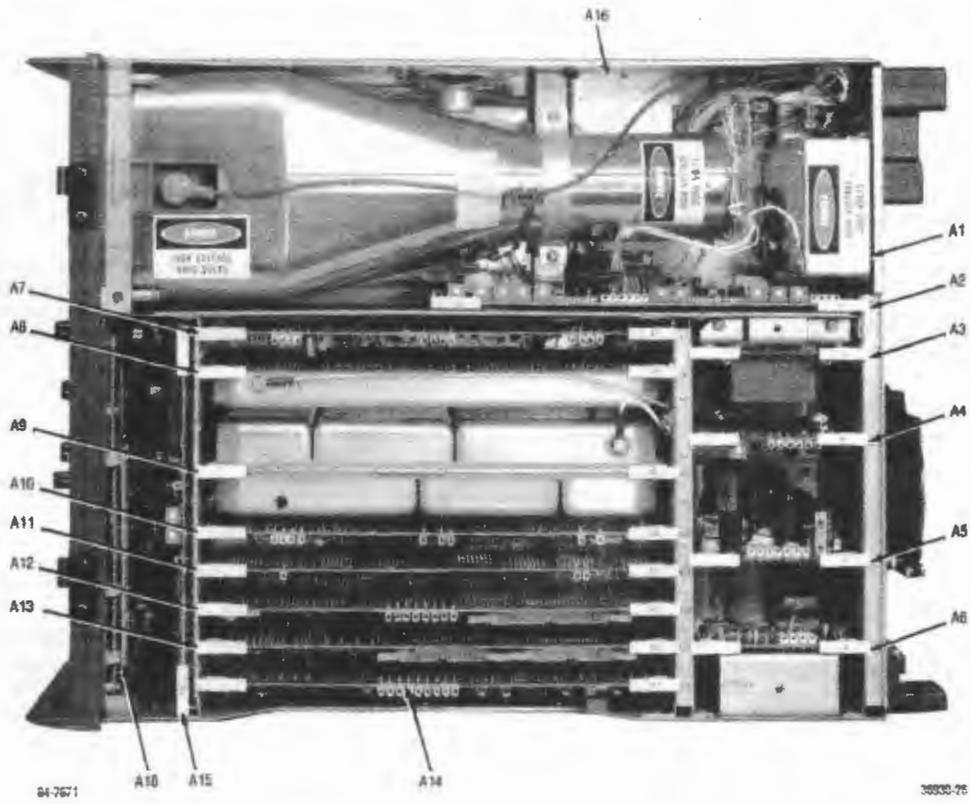
Figure 1-5. Communications System Analyzer — Top View, Cover Removed
