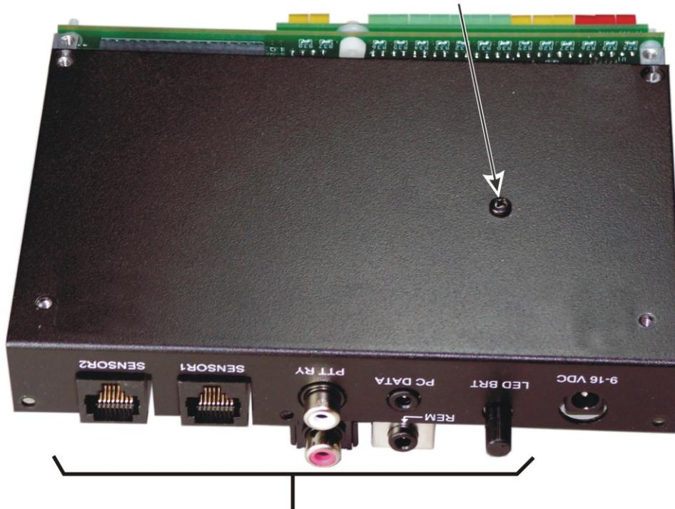
① REMOVE THE SCREW YOU PLACED THROUGH U3 TO HOLD THE SPACER AND SLIDE THE BOTTOM COVER ON FROM THE REAR, FITTING THE LED BRIGHTNESS CONTROL AND CONNECTORS THROUGH THE OPENINGS IN THE COVER.
