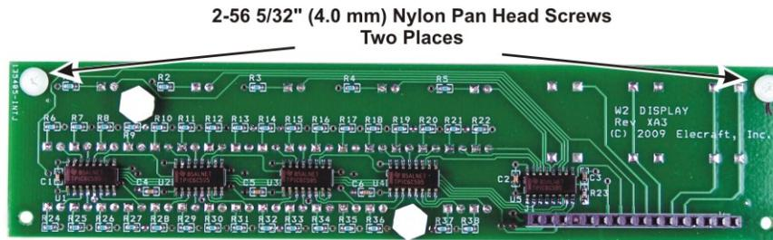
Figure 3. Nylon "Bumper" Screws in Front Panel Board.
