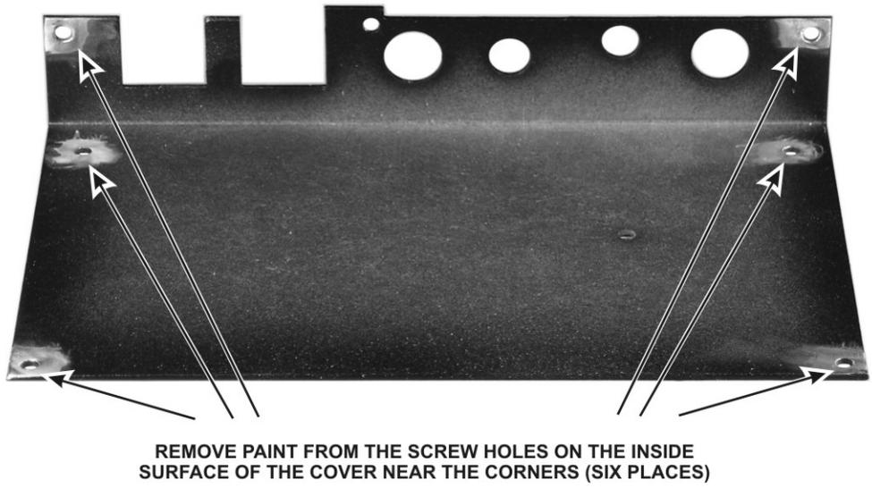
Figure 6. Preparing the Bottom Cover for Mounting.
