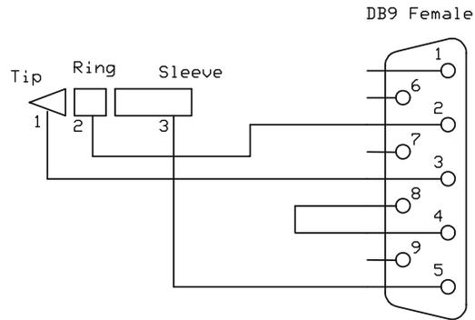
Above is the schematic diagram of the optional RS232 serial interface cable. A kit of parts to assemble the cable is available from Elecraft (order W1SERKT), or you can order a factory-assembled cable from Elecraft (order KXSER). If you order the KXSER cable, it may arrive in a bag marked E850369.
