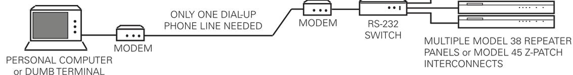
The best way to control a Model 38 over a phone line is with an RS-232 terminal and a pair of modems. If you have several Model 38s at a common site, use a multiport RS-232 switch so you don't have to obtain multiple phone lines.
