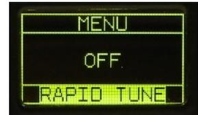
With the cursor in the 100 Hz position, after 'X' rotations of **[T]**, the cursor automatically moves to the 1 kHz position until rotation stops. Then the cursor returns to the 100 Hz position to allow for fine-tuning.
