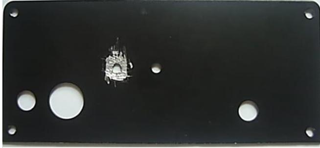
2. Before install Q10, please scratch the install position on the back cover to Q10 has a good surface contact.
