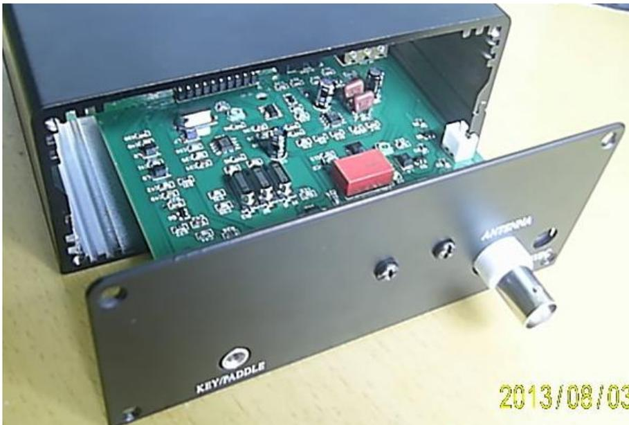
Secure the back cover with screws, put studs on the display board and then secure the front cover. Install two knobs, assemble finished.
