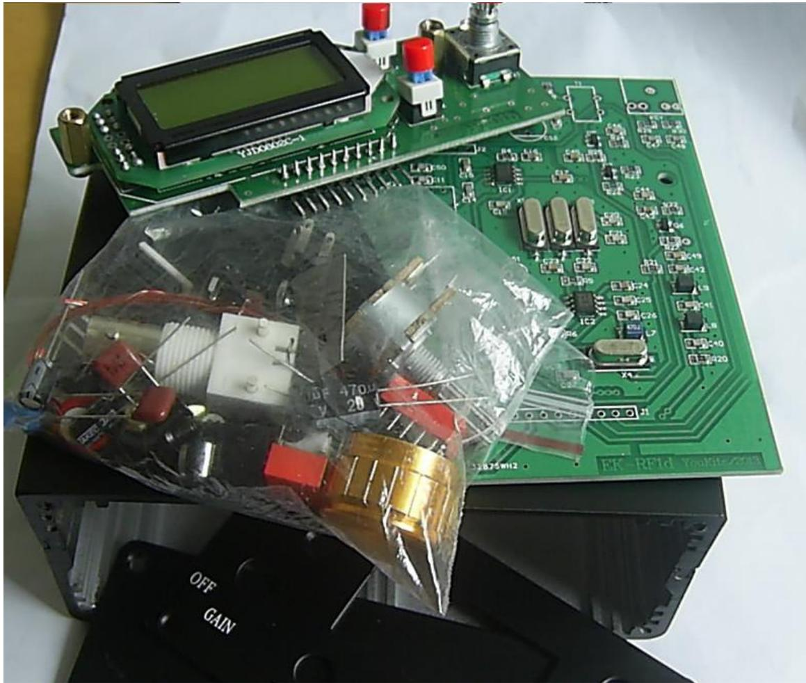
EK-1B 3 Band CW QRP transceiver kit is easy to build, it has SMD finished by the factory. There are 2pcs of PCB, the main board and display board. To guarantee the building success, the display board and main board have been assembled and tested including the MCU, LCD and DDS.
