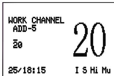
Press **▲** or **▼** key to change the selected channel, and press **(ENT)** key to accept. Then press **◀** or **▶** key to enter the next channel.
