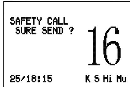
Press the **(ENT)** key again to make the call, or press **(CLR)** to cancel. When the call is sent, the radio will be set to the working channel. Allow a few seconds for the stations receiving the call to switch to the working channel. Then make a normal voice call on the selected working channel.
