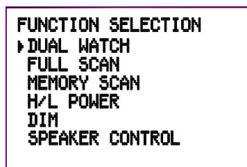
Press the **▲** or **▼** key to move the cursor to the required function (DUAL WATCH, FULL SCAN, MEMORY SCAN, H/L POWER, DIM or SPEAKER CONTROL), then press **(F)** key to confirm. When the desired function is selected, the relevant screen will be displayed. Press **(F)** key again to restore normal operation, and press **(CLR)** key to change to the main screen.
