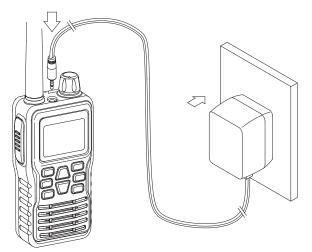
**Note:** The Ni-MH batteries and AC adapter are the optional accessories of the radio. The charging can not stop itself without prevention even when the batteries have been fully charged. Do not forget to remove the adapter from the radio when the radio is fully charged.
