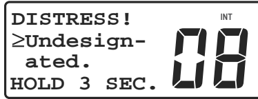
Distress Alert Screen
