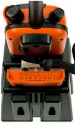
Figure 8 Emergency battery in the storage bay
