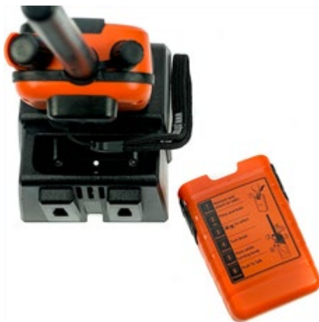
Figure 7 Tron TR30 radio in the charging bay
