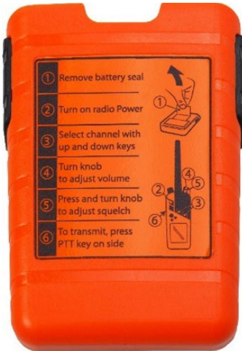
Figure 4 Tron TR30 Emergency battery (orange)
