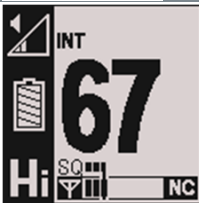
Figure 10 Noise cancel (NC) symbol on VHF screen (bottom right)
