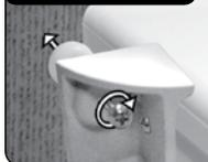
2. Insert the transceiver into the opening.
