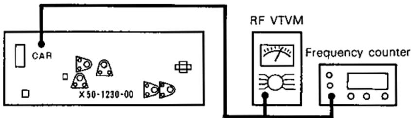
FIG. 5 CARRIER OSCILLATION ADJUSTMENT
