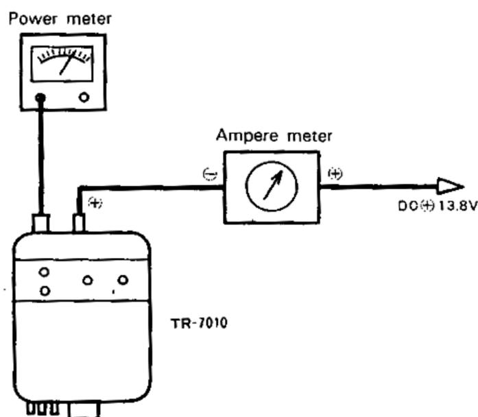
FIG. 9 CONNECTION OF AMPERE METER
