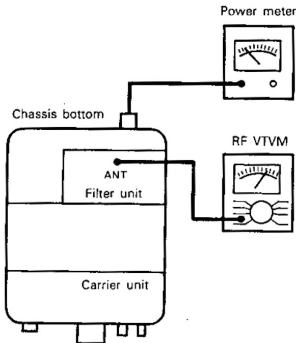
FIG. 11 ADJUSTMENT OF CARRIER SUPPRESSION
