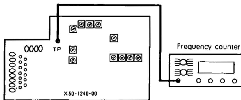
FIG. 4 41MHz OSCILLATION ADJUSTMENT
