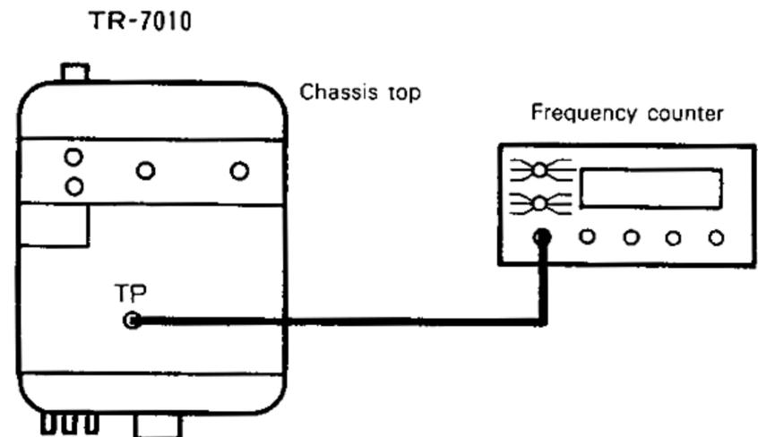
FIG. 1 ADJUSTMENT OF 8MHz FREQUENCIES
