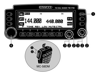
Switch the DC power supply ON, then press the PWR switch.
