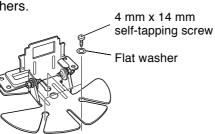
4 Position the grooves on the front panel over the bracket tabs.
