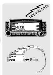
This transceiver provides the following scan types, plus Visual Scan {page 45}. Visual Scan graphically and simultaneously shows how frequencies in a specific range are busy.
