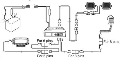
**Note:** Always connect the 4-pin plug on the modular plug cable supplied with the transceiver to the front panel.
