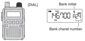
(4) To return to a regular memory channel, rotate [DIAL] while holding down [BAND], or repeatedly push [BAND].
