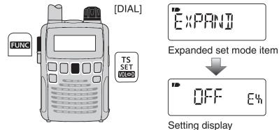
(4) While holding down [FUNC], rotate [DIAL] to select "ON."
