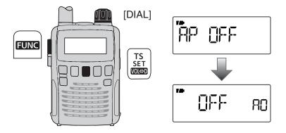
③While holding down [FUNC], rotate [DIAL] to select a desired time or to turn the function OFF.
