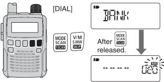
• After releasing [MODE], "-- -- --" is displayed instead of the frequency display, and only the "MR" icon blinks.
