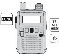
➡ While holding down [FUNC] and [TS], turn the power OFF, then ON again to partially reset the receiver.
