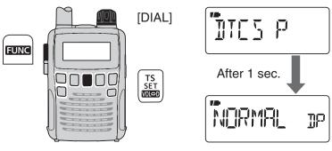
(5) While holding down **[FUNC]**, rotate **[DIAL]** to select the polarity from normal (NORMAL) and reverse (REV).
