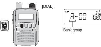
(5) Rotate [DIAL] to select a desired bank channel number.Only vacant bank channel numbers are displayed.
