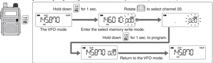
[EXAMPLE]: Programming 145.870 MHz into memory channel 20 (a blank channel).
