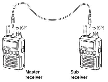
**NOTE: DO NOT** push any key on the sub-receiver during cloning. This will cause a cloning error.
