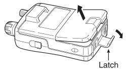
2 Install 2 R6 (AA) size Ni-MH batteries.
