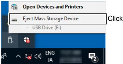
5. When “Safe To Remove Hardware” is displayed, disconnect the USB cable from the PC.
