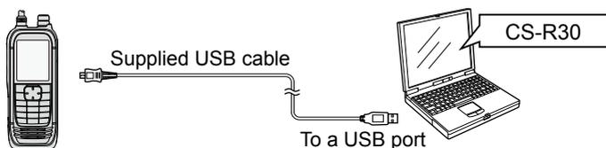
By using the CS-R30 CLONING SOFTWARE and the supplied USB cable, you can clone with a PC.
