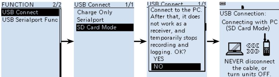
**TIP:** You can also read or write the data using the microSD card and a card reader (user supplied), without a USB cable. Remove the microSD card that contains the data from the IC-R30, then read it on the PC using the card reader.
