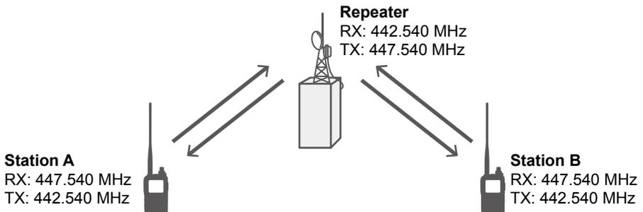
Reverse the RX/TX frequencies and titles. The arrows FROM the transceivers to the repeater are transceiver TX and the arrows FROM the repeater to the transceiver are transceiver RX.
