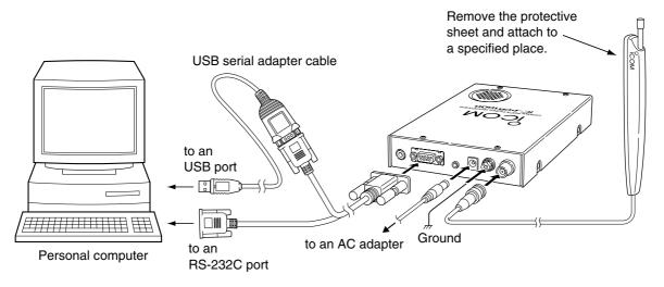
\* When using the USB serial adapter cable, USB serial port can be used. It is necessary to USB driver installation. The driver is supplied with the USB serial adapter cable.
