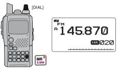
②Push and hold [S.MW](MR) for 1 sec. to enter select memory write mode. ③ Push [▲](2) or [▼](8) several times to select "SKIP."
