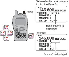
⑥Push [S.MW](MR) for 1 sec. to erase/transfer the bank contents.
