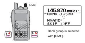
(5) Rotate [DIAL] to select the bank group (from "A" to "Z") or bank channel number (from "00" to "99").
