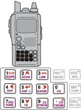
Depending on the tuning step setting, it may not be possible to input a 1 kHz digit. In this case, enter "0" as 1 kHz digit, then rotate **[DIAL]** to set the desired frequency.
