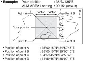
When the target position enters the area as above, the GPS alarm will sound.
