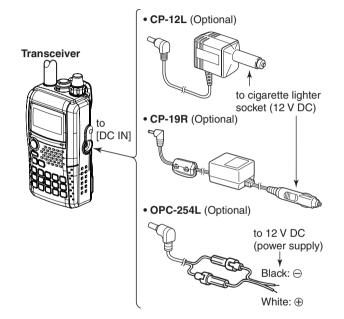
**NOTE:** Up to 5 W (approx.) of maximum output power is available when using external DC power. However, when the supplied voltage exceeds 14 V, the built-in protection circuit activates to reduce the transmit output power to 2.5 W (approx.).
