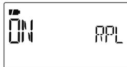
**NOTE:** When Auto reply is “ON,” the power save function (p. 125) is disabled to receive call sign signal properly.
