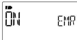
**NOTE:** The EMR communication function is turned OFF automatically when turning transceiver's power OFF
