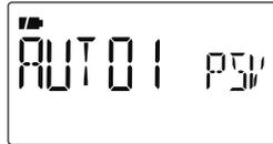
**NOTE:** Power save function is disabled when using the external power supply (more than 10 V DC) or if the Auto replay function is set to ON (p. 132).
