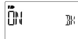
**NOTE:** The break-in function is turned OFF automatically when turning transceiver's power OFF.
