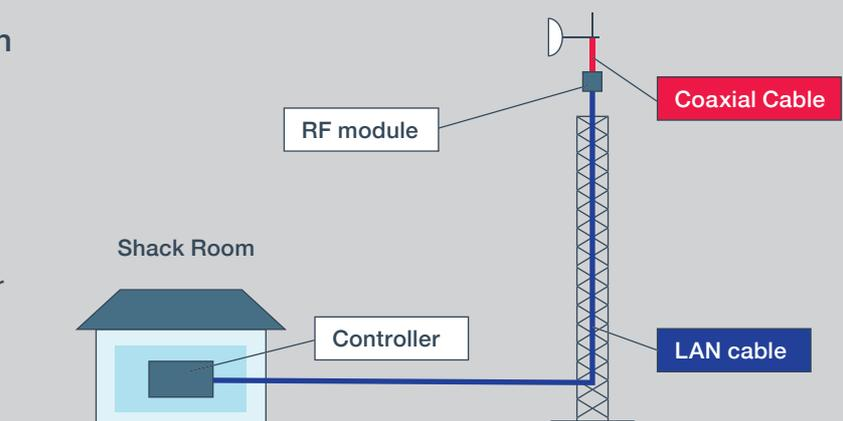
A LAN cable is used to connect the controller to the RF module. By using this kind of cabling set up, only a small length of a coaxial cable (about 30-40 cm) is required between the RF module and the antenna. Thus, only minimal loss occurs. For example, even if the controller and RF unit are separated by 30 meters, the loss from coaxial cable is still minimized, due to the short coaxial cable length.
