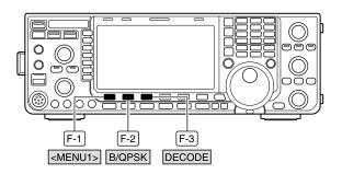
• PSK decode screen— the BPSK mode
