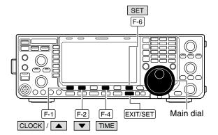
The IC-7600 has a built-in calendar and 24-hour clock (accuracy ±75 sec. per month) with daily power ON/OFF timer functions. Before operating these timer functions, set the current date and time.
