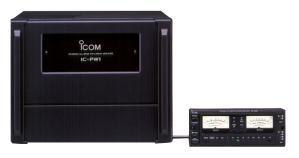
Full-duty 1 kW linear amplifier including an automatic antenna tuner. Has automatic tuning and band selection capability. Full break-in (QSK) operation is possible. The amplifier/power supply unit and the remote control unit are separated.
