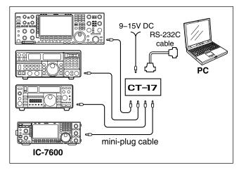
When the transceiver is connected to a PC with the USB cable (purchased separately), the optional CT-17 is not required.
