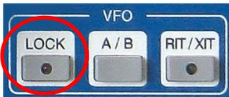
All controls that will have an effect on the frequency selected can be locked through pushing **LOCK** button which is located in the cluster VFO.
