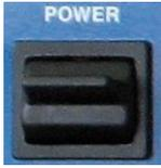
Switch off the PT-8000A by POWER switch and restart after a waiting time of about 10 seconds.
