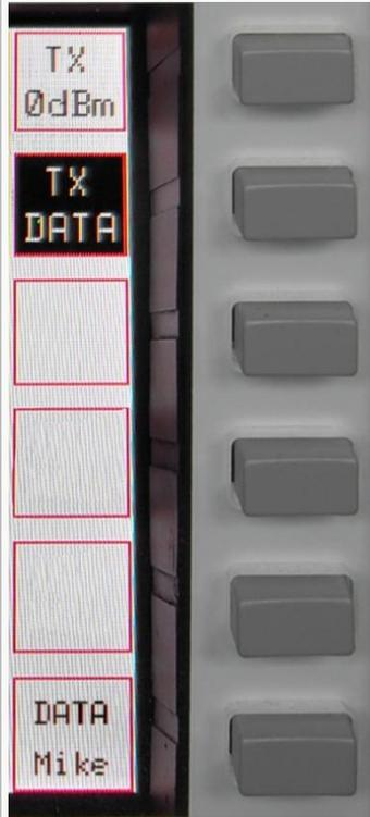
In case this softkey is activated (the softkey will be displayed inverse; **DATA**-LED will turn on) the signal at the 0dBm input (MIC-PTT Pin 4) will be transmitted when PTT is switched.
