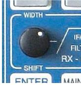
Adjustment of EQ bands is also possible with WIDTH/SHIFT control (as long as the EQUALIZER menu will be displayed and EQ is activated):
