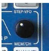
Pushing softkey **BANK 1**, **BANK 2** and **BANK 3** gives access to the banks. Use MEM/CH / STEP-VFO to select desired memory channel (0 ... 99).
