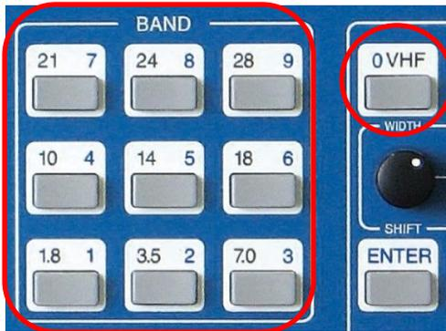
Pushing a band pushbutton selects one of two stored frequencies within the desired band (see Table 13 and 14).
