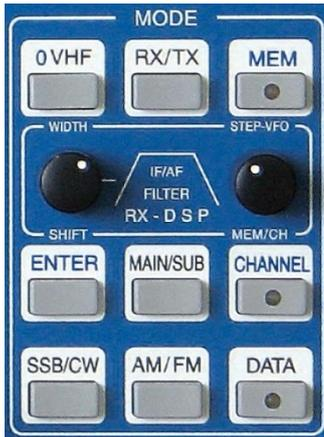
Pushing **MEM** button located in the cluster MODE will store the frequency and additional VFO values of the active RX to one of the 297 memory channels organized in three banks with 99 memory channels each bank.
