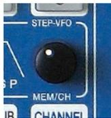
After selecting the memory bank through pushing softkeys **BANK 1**, **BANK 2** and **BANK 3** the control MEM/CH / STEP-VFO gives access to 99 memory channels by turning.
