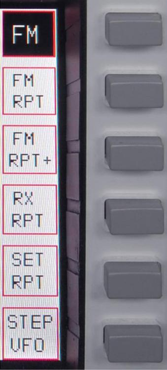
Frequency Modulation (standard mode); the softkey will be displayed inverse (as shown here); the display will show **FM** (left of frequency).
