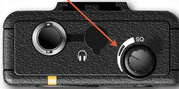
Figure 9 - Recommended squelch setting range.
