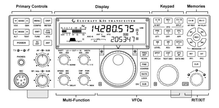
**Primary Controls (pg. 13):** These controls provide basic transceiver setup, including power on/off, band, operating mode, AF and RF gain and squelch, ATU and transmit controls, display modes, and menus.
