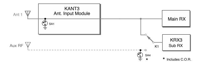
Figure 1. Basic Main/Sub Receiver Routing (no KAT3A)
