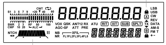
**Filter Graphic:** This shows the approx. bandwidth and position of the receiver's I.F. passband. See **Filter Passband Controls**, pg. 25.
