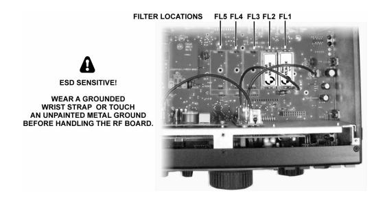
There may be a mix of 5-pole filters (below left) and 8-pole filters (right).
