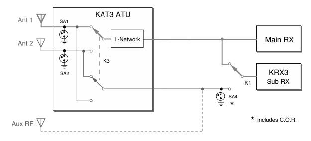
Figure 3. KAT3A ATU Antenna Routing
