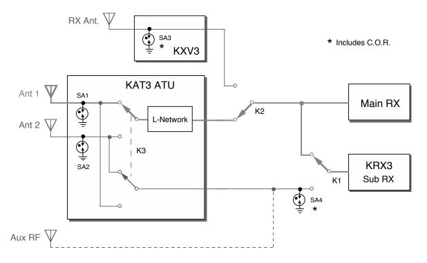
Figure 4. Complete Main/Sub Receiver Antenna Routing
