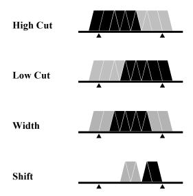
filter passband controls don't apply in FM mode. SHIFT control granularity can be set to either 10 or 50 Hz in CW and DATA modes; see CONFIG:PB CTRL. In Sync AM mode (AM-S), SHIFT selects the upper or lower sideband.
