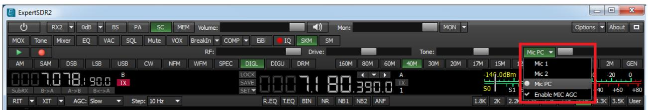
Figure 4.4 – Choose the microphone connected to PC
