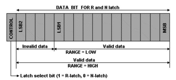
R packet is 16-bits MSB first hold the R Value, 1 Control Bit always signal that it is a R packet, then LE is toggled to complete this packet.
