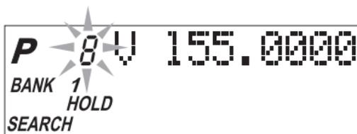
2. Turn the VFO control clockwise to move up the frequency step, and turn the VFO control counter-clockwise to move down the frequency step.
