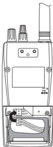
7. Replace the Battery Cover by putting the two tabs in the corresponding opening and sliding it upward until it locks in place.
