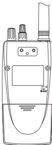
3. Press in on the ribbed area and slide the Battery Cover down and off.
