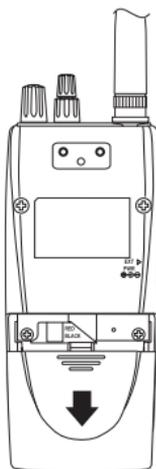
4. Carefully unplug the Battery pack and lift it out of the case. You may need to exert slight pressure toward the top of the scanner as you slide the Battery Pack out of the case.
