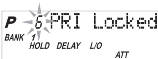
You can also remove **L/O** from all “Locked Out” channels in the selected Scan Banks (those appearing on the display.) Press and hold **(L/O)** for at least 2 seconds. You will hear 2 beeps and all channels except empty channels (000.0000MHz) are returned to the scanning cycle in the selected Scan Banks.
