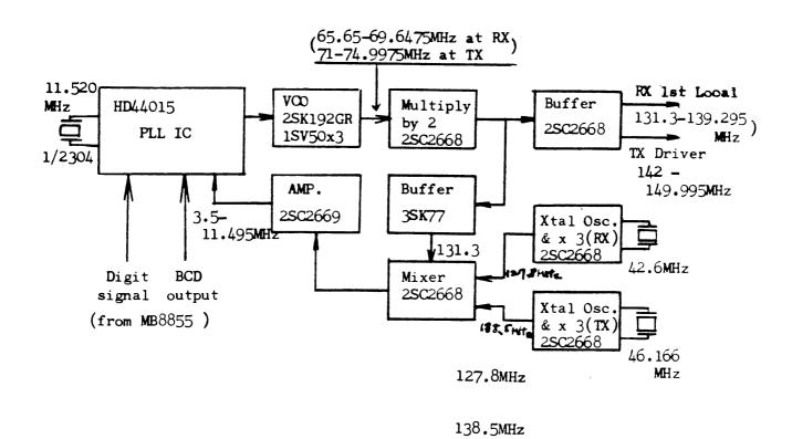
The PLL IC HD44015 is functionally comprised of Phase Detector, Low Pass Filter, Programmable Divider and Divider for reference frequency.
