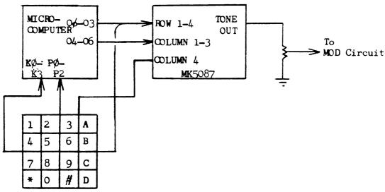
16 keys on the keyboard will be so changed by the microcomputer as to serve as these for DTMF. (Note this is available only for the U.S. version unit. The European version unit does not include tone encoder IC MK5087 and its peripheral circuits)
