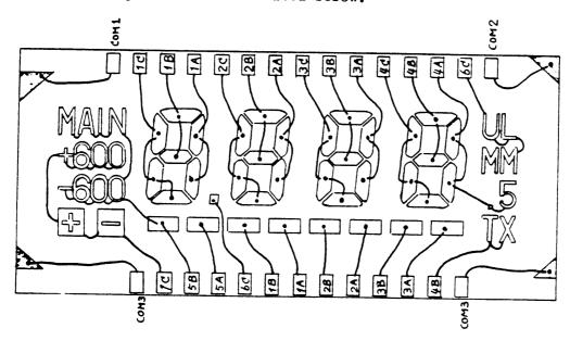
The LCD unit terminal pin numbers like 1C, 5B, .... correspond to those of the LCD driver IC TPO401 pins.
