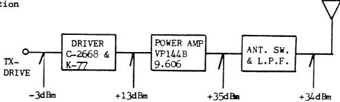
The PLL output (TX Drive) signal, which is put out in the range of 142.000 through 149.995MHz, is directly amplified without being mixed to get an output of more than 2.5W. The output is rectified by the voltage doubler rectifier circuit to obtain DC voltage and then A/D-converted at the control section so that the microcomputer functions to light up an RF meter. The DC voltage thus obtained controls the 2nd gate of the K-77 driver FET to obtain the lower power of 0.6W.
