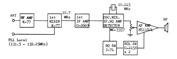
The incoming signal is RF-amplified by 3SK77 and then mixed down (by K77) with the PLL local output to get the 1st IF of 10.7MHz. The 10.7MHz signal is then amplified by C-2669 (1st IF AMP) and fed into MC-3357 where it is mixed with the 2nd local output of 10.245 to produce the 455kHz, 2nd IF and then demodulated to drive a speaker by and through AF amplifier IC M51182L.
