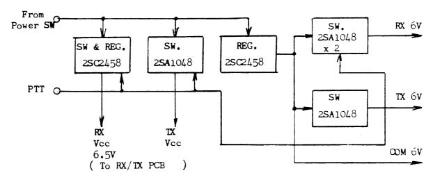
6V DC for oscillation circuit provided in the PLL circuit and also for receive is fed through regulator circuit. But the transmit power stage has only a switch circuit. So, RF output power is varied depending upon the change of power supply voltage. In other words, the output power largely changes when operating the unit immediately when battery is fully charged or when it comes near to its discharging end. Pressing the PTT Switch will turn TX/Vcc On and turn Off RX/Vcc 6.5V.
