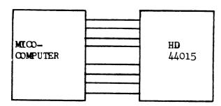
4-bit parallel signal (N $\phi$  - N3, N3 $\pm$ MSB) is transferred from the microcomputer to the PLL IC HD44015 one after the other in the form of digit signal (D $\phi$  - D3, D $\phi$ =1st digit).
