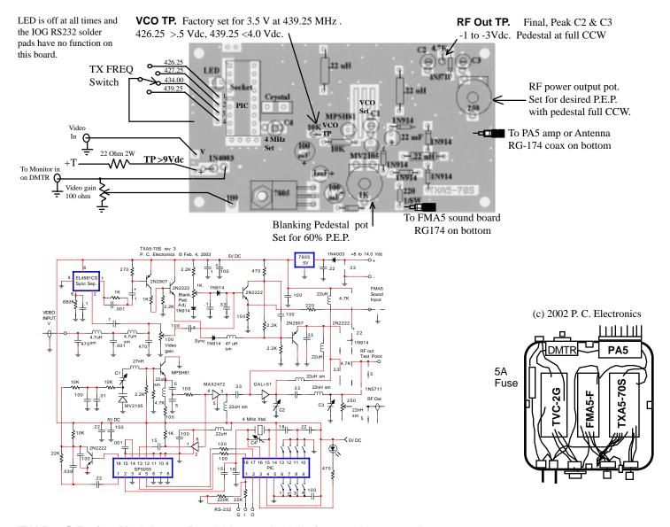
TXA5-70S Exciter Modulator - Read this completely before touching any adjustments.
