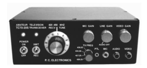
The TC70-20S transceiver is designed to provide over 20 Watt p.e.p. (sync tip), continuous duty, of AM video modulated RF in the 70 cm (420-450 MHz) Amateur band in transmit, and downconvert the whole band to TV channel 3 (61.25 MHz) or 4 (67.25 MHz) to enable receiving on any standard NTSC television set or VCR with a tuner.
