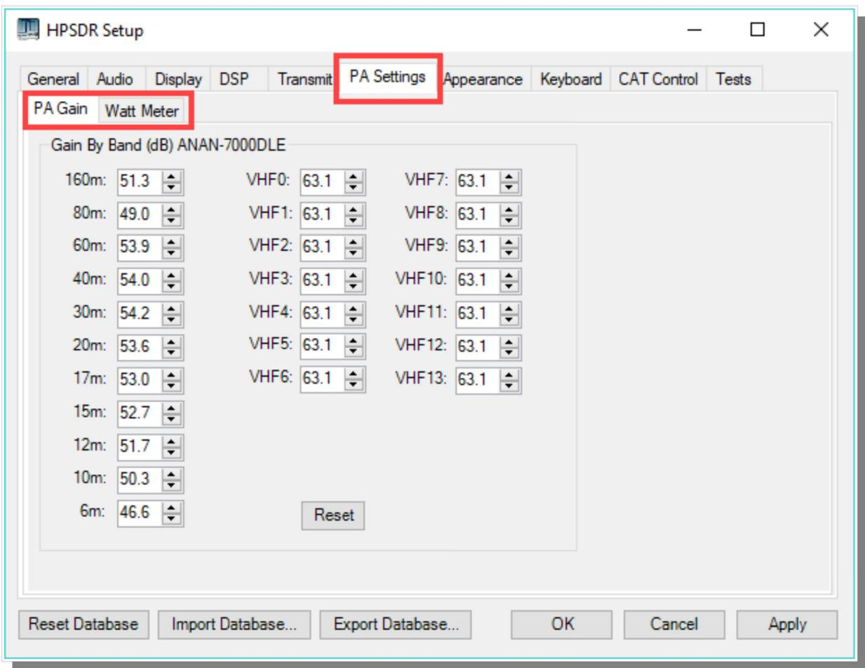
Use the following manual calibration procedure to properly set/calibrate your ANAN-7000DLE power output into a dummy load:
