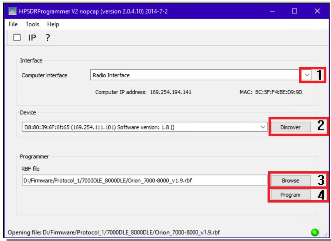
1 – Choose the **Computer Interface** that the radio is connected to using the pull-down menu.
