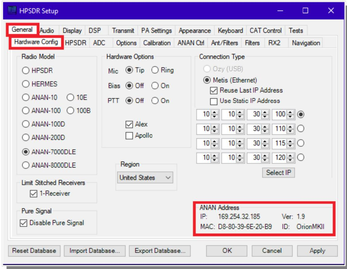
Go to → GENERAL → Hardware Configuration tab and note the IP Address and MAC address that are read from the radio's flash memory.
