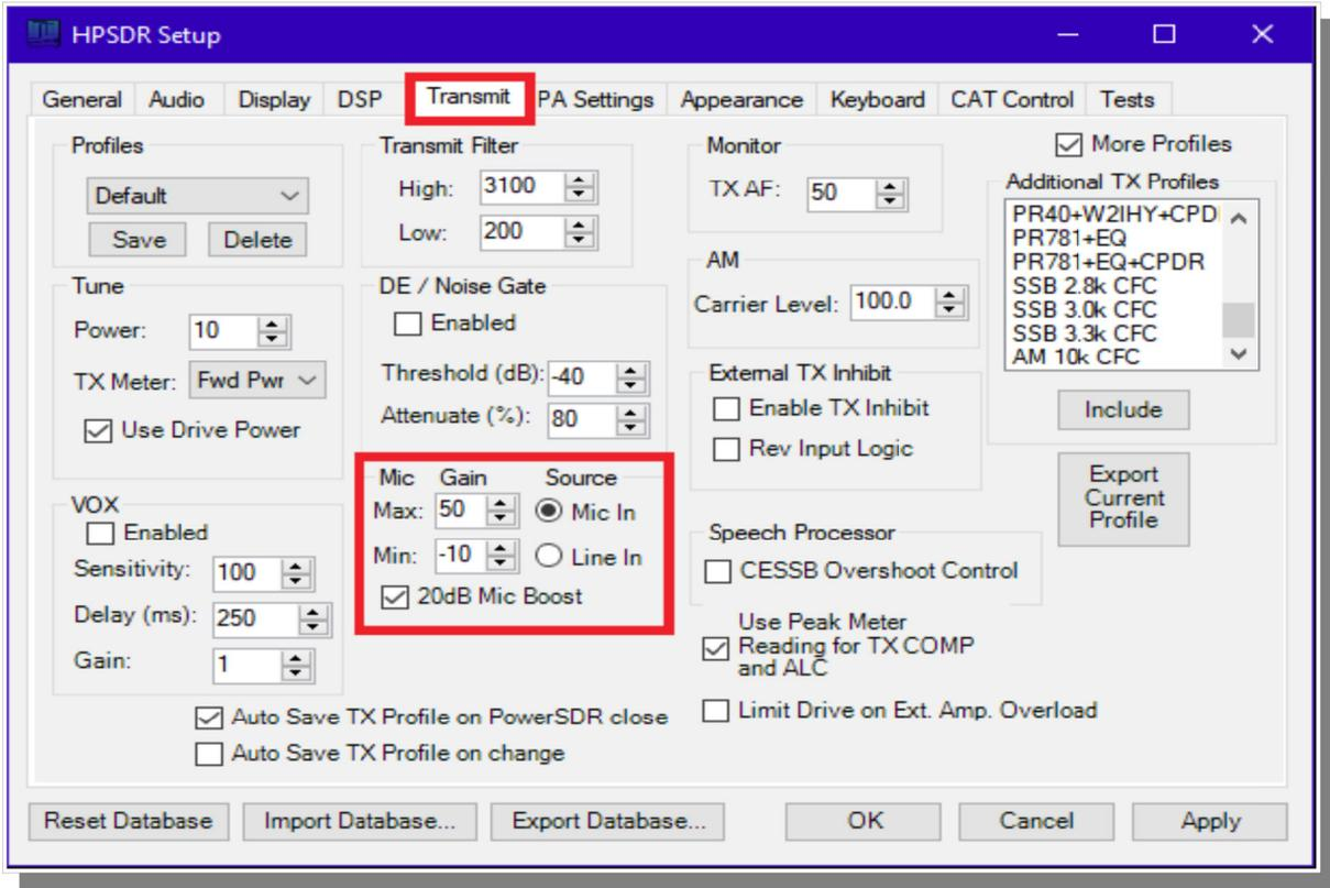
If 0 dB voice peaks cannot be achieved with the slider at the extreme right, go to the Setup, transmit tab [lower left], check **"20db Mic boost"** and readjust the "MIC" gain control on the console for 0 dB on voice peaks.
