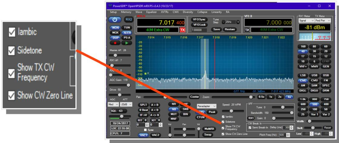
Note that you can see your CW [BFO] CENTER FREQUENCY or TX FREQUENCY by checking the boxes on the console. Those convenient vertical yellow marker-lines are really great when you are working split. The SPEED of the internal Iambic Keyer is shown at the top of this picture.
