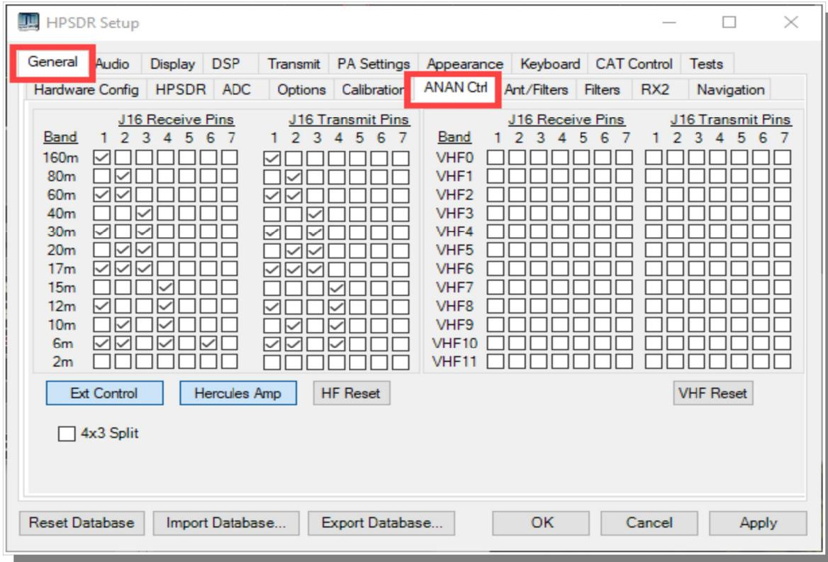
4x3 Split – When enabled the 7 OC outputs are split into 1x4 and 1x3. The first 4-bits are controlled by VFOA band data and the upper 3 are controlled by VFOB band data.
