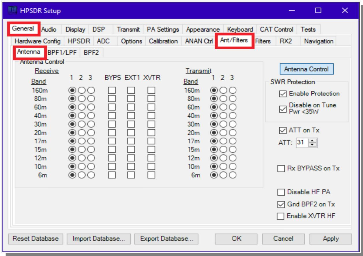
Separate receive and transmit antennas can be selected by use of the 1,2,3 radio buttons. This corresponds to the ANT1, ANT2, and ANT3 ports on the rear panel. Receive only antennas can be connected to the 'Rx BYPASS' or 'EXT1' ports on the rear panel. The 'Rx BYPASS' port does not have a BPF in the receive chain. The 'XVTR' port is for use with a transverter. When the box is checked the 'XVTR' port will only be switched when a VHF band is active.
