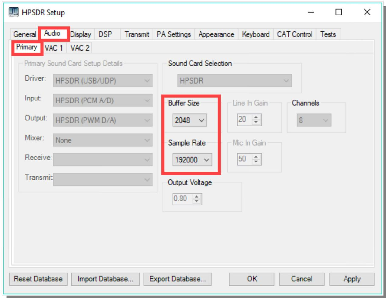
The appearance of the Panadapter can be adjusted with the **ZOOM** settings, **Sample Rate**, and **SETUP --> DISPLAY --> RX1 [or RX2] --> Fast Fourier Transform Size [min to max] Bin width**.
