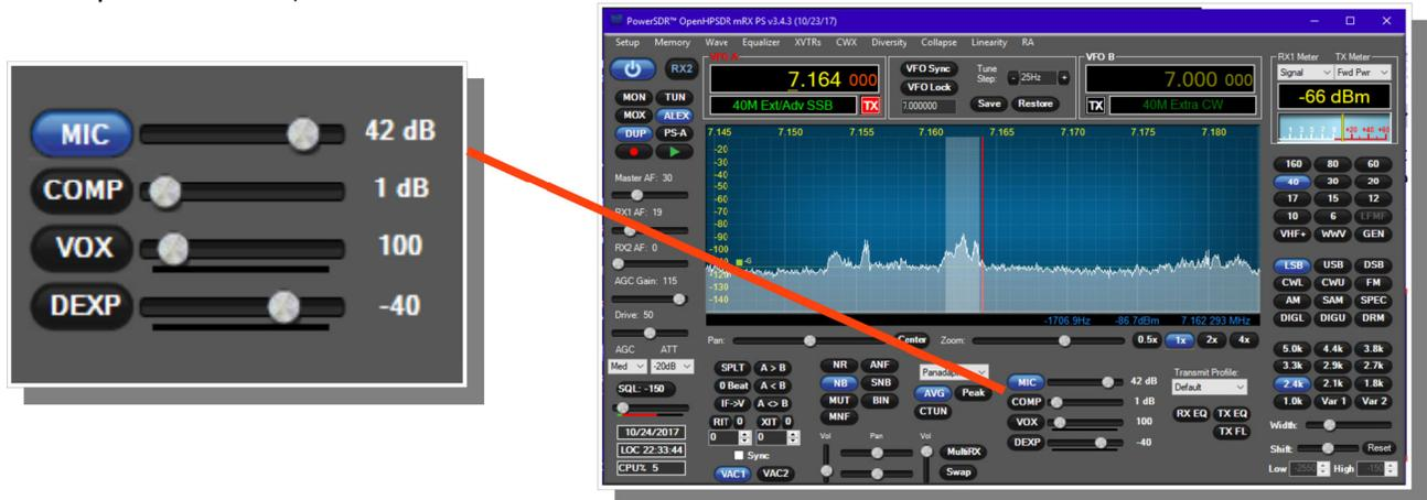
Locate the "MIC" gain control slider. It is located at lower right, below the panadapter. The present mic gain setting is shown just to the right of the MIC gain slider.
