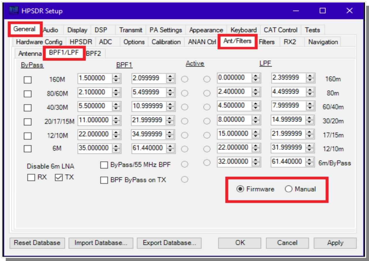
**When under firmware control the BPF and LPF are automatically selected as you change bands. Manual mode must be selected for any of these controls to function.**
