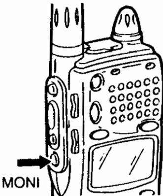
If the received signal is weak or intermittent, press the **MONI** key. While the **MONI** key is pressed, the squelch is unmuted, and the signal will be easier to hear.
