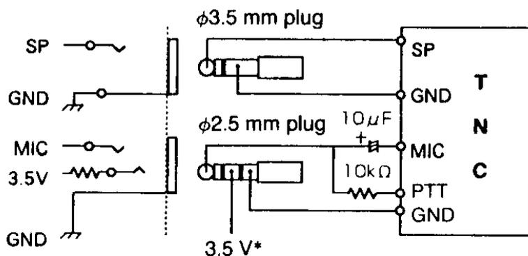
\*Power is supplied from the internal 3.5 V line through a 100  $\Omega$  resistor.
