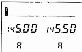
During VFO mode, hold down the **F** key and press the main band's band key. Each press of the key switches the transceiver between the UHF and VHF bands.
