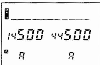
With the L band sets to the **MAIN** band, and the transceiver in VFO mode, press the
