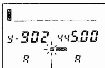
An alarm sounds, **P** flashes on the display, and the transmitting station's code is displayed.
