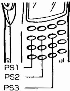
Press one of the <sup>PS1</sup>4, <sup>PS2</sup>5, or <sup>PS3</sup>6 keys in VFO mode. When the VFO band and the programmed scan band are different, the transceiver switches to the programmed scan band and starts scanning. The display and operations are the same as for band scan. "P1, P2 or P3" flashes during scan.
