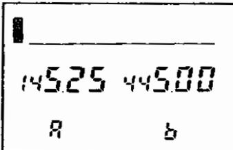
Set the frequency for the main band. Switch the main band and sub band, and set the frequency for the other band.
