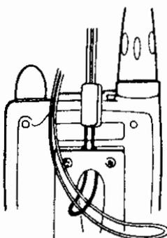
Attach the hand strap between the belt clip and the groove on the back of the transceiver.
