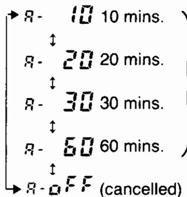
APO appears on the display. If no operations are performed within the specified time the transceiver turns off. 30 seconds before it turns off, the APO icon flashes, and the alarm sounds.
