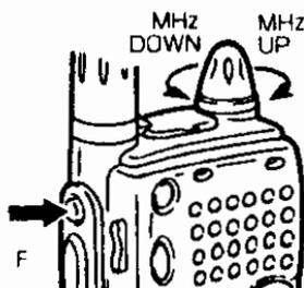
Press and hold the **F** key down and rotate the **DIAL**.
