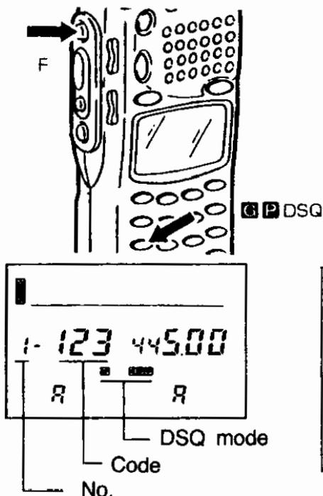
DSQ only operates on the main band. The sub band DSQ setting is not displayed, and the DSQ setting display always refers to the main band side.
