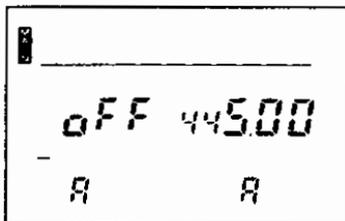
Press the **PTT** key to transmit when offset or split is set (for the transmission display will change). If the transmission frequency is outside the allowed transmission frequency range, **OFF** is displayed when you press **PTT**, and no transmission takes place.
