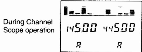
For each band, the signal strengths of five channels around and including the center frequency (marked with ▼) are displayed vertically.
