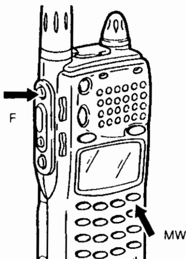
Hold down the F key and press the
