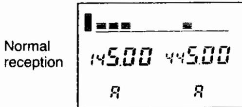
The signal strength of the displayed frequency is displayed horizontally.
