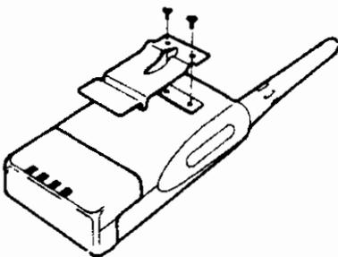
Attach the belt clip to the back of the transceiver using the two screws provided as shown in the diagram on the left.
