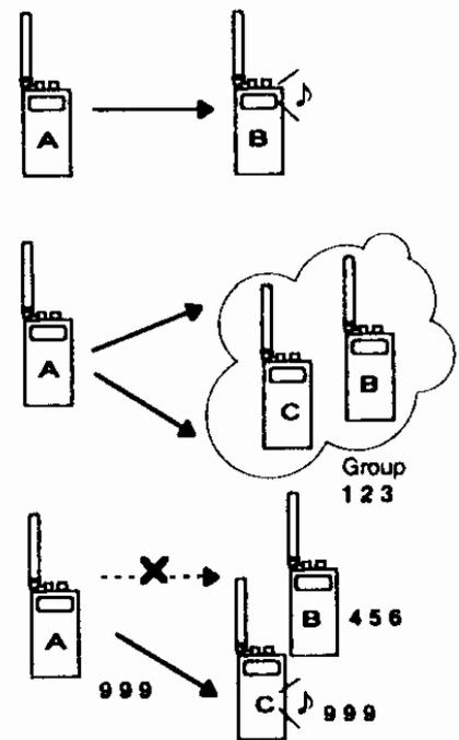
There are three types of DSQ code, all of which consist of three numerical digits. DSQ codes can be independently set for both the L and R bands.
