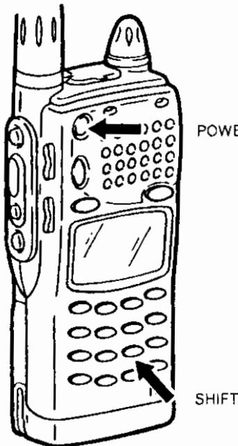
① Hold down the
