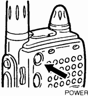
Press and hold the **POWER** switch down for a short time.
