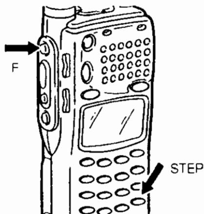
① In VFO mode, hold down the **F** key and press the
