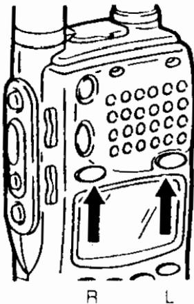
Press the sub band key (the key on the side that **M** is not displayed).
