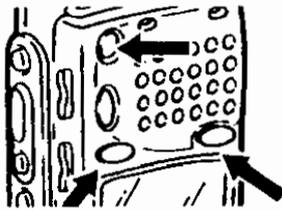
Hold down a band key (L or R), and turn the power on.
