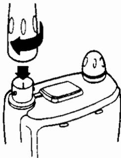
Hold the antenna by its base, and align the grooves in the connector at the base of the antenna with the protruding guides on the transceiver's antenna connector. Slide the antenna down and turn it clockwise to lock it into place.
