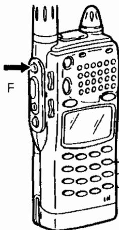
Hold down the F key and press the
