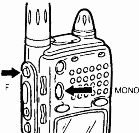
Press the **MONO** key while holding down the **F** key.
