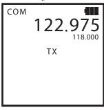
Release the PTT to end the transmission and the SP-400 will once again receive the selected COMM frequency. If the optional Headset Adapter is being used, the SP-400's internal microphone will be deactivated and the microphone on the headset may be activated by either pressing the SP-400's PTT or pressing an inline, remote PTT.
