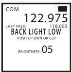
Once in the low back light mode, the back light can be further adjusted from level 0 to level 10 by pressing the up or down keys.
