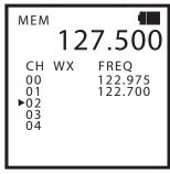
The first available memory channel will be displayed with an arrow on the screen. Now press either the Up or Down Key to scroll through the 20 memory channels. If a memory channel is already storing a frequency, the stored frequency will be displayed next to the memory channel number on the screen while your selected frequency remains on the top line.
