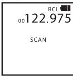
When a broadcasting signal is found, the word SCAN will flash and the SP-400 will stop temporarily on that frequency. If the broadcasting signal is cut off for more than two seconds, the Scan will resume until another signal is found.
