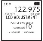
The contrast can be adjusted by pressing the up or down keys. Press the clear key to save the setting.
