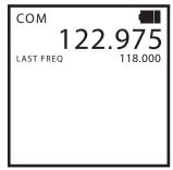
From the example above, the SP-400 is receiving 122.975 MHz with the last frequency being 118.000 MHz. To manually enter a desired frequency such as 118.700 MHz, enter 1 1 8 7 0 0 using the numeric keypad. As each digit is entered, the flashing cursor moves to the next digit. Six digits may be required to select a frequency.
