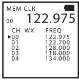
The first five memory channels with stored frequencies will be displayed on the screen. Press the Up or Down Key to scroll through the memory channels to select the memory channel to clear. Once the desired memory channel is displayed, press the Memory Clear Key (also the 0 Key on the Numeric Keypad) to clear the selected channel. Additional channels may be cleared by once again pressing the Up or Down Key to make another selection and then pressing the Memory Clear Key.
