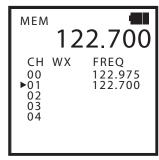
You may also overwrite an existing memory channel or select an available memory channel other than the first one displayed. Once again, select the desired frequency and then press the Memory Key.
