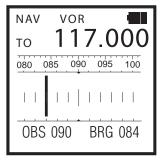
The three digits in the lower left-hand side of the screen are the Omni Bearing Selector (OBS) setting. Whenever the CDI needle is centered, such as when a VOR signal is first received, the OBS setting represents your bearing to or radial from the selected VOR station. The TO or FROM next to the frequency specifies whether the OBS setting is a bearing to or a radial from the VOR.
