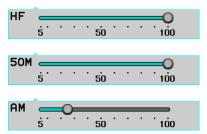
The maximum transmit power that can be set is less than or equal to the following MAX POWER set in the transceiver set mode.
