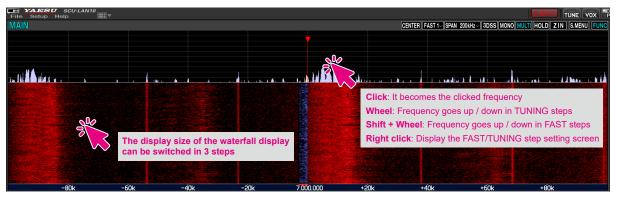
If you hold down the [SHIFT] key on the keyboard and turn the mouse wheel, the frequency will increase or decrease in FAST steps.
