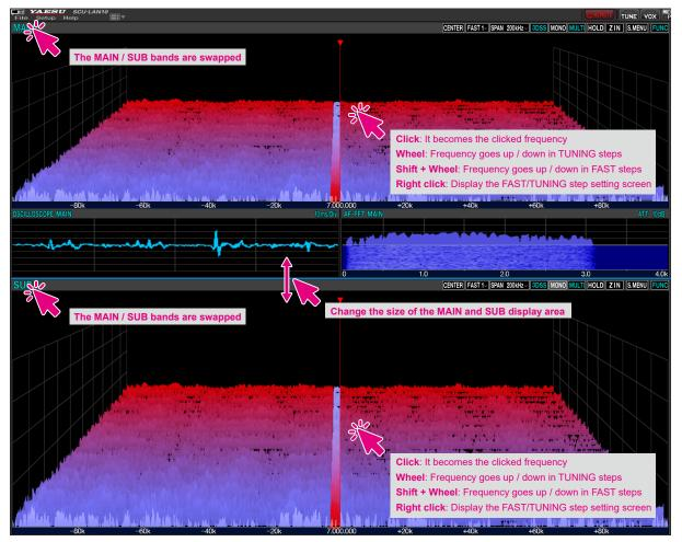
If you hold down the [SHIFT] key on the keyboard and turn the mouse wheel, the frequency will increase or decrease in FAST steps.
