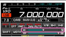
Turn the **mouse wheel**, or drag or click on the slide bar to adjust the receive audio to a comfortable volume.
