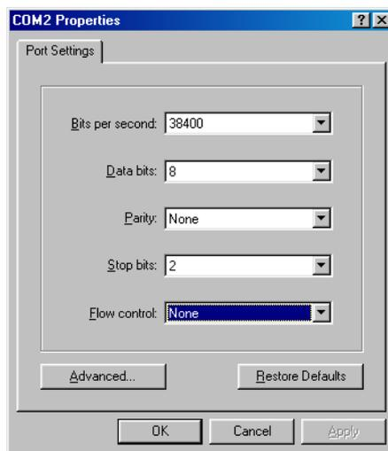
Set 'Bits per second' to 38400, set 'Date bits' to 8, set 'Parity' to None, set 'Stop bits' to 2 and set 'Flow control' to None. Click OK. *Remember, a PC of at least 486DX266 will be required for reliable transfer at 38400bps.*
