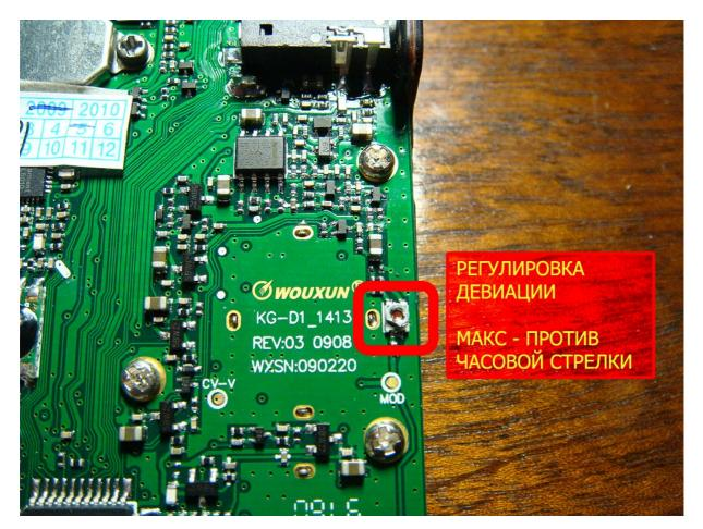
7. Adjust deviation according to your needs. I recommend to set MAX deviation (turn the trimmer counterclockwise until modulation disappears, than turn back a little bit to catch maximum deviation position).
