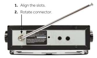
Your scanner's frequency sensitivity depends on its location and the antenna length. For best reception, adjust the antenna's length as follows:
