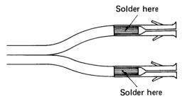
3. Insert the pins into a supplied connector housing observing proper polarity so that the pins are fixed in the housing by the barbs of each pin.
