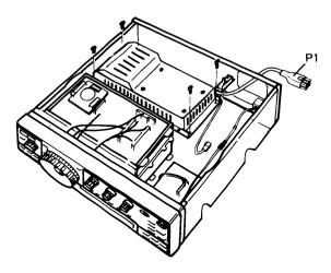
3. Pass the DC power cable attached P1 through the hole of the AC power socket plate as shown in the illustration, then insert the bushing into the hole.
