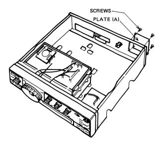
2. Put the power supply unit into the set so that its cables are toward the rear as shown in the illustration, and attach it to the chassis by the supplied screws.
