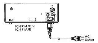
3. By turning the transceiver power switch ON, this unit will be turned ON and supply a 13.8V DC to the transceiver.
