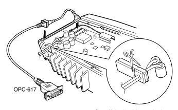
Cut off the bushing as in the illustration, when you install the optional OPC-617.
