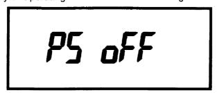
If you press the "▲ or ▼" button in this setting mode, power save On/Off will toggle on the LCD.
