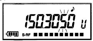
Press the "FUNC + ▲" button, the fifth digit of the frequency display will start to flash. Now press "▲ or ▼" button to set the value to " 6 ":
