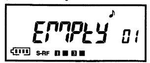
If only one channel will remain due to the skipping of channels from the scanning process, the process will stop and "EMPTY" message will appear on the LCD.
