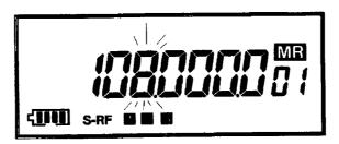
When frequency selection has been made, to store in to memory, press the MR (MW) or "MON" button.
