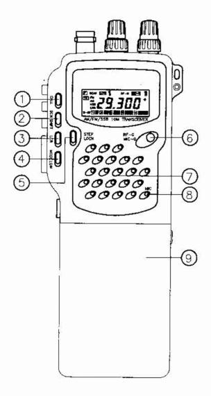
1. Call: For Call monitoring on call frequency 29.300MHz, just press "CALL". 29.300 flashes appears on the display, and the transceiver stays on all frequency 29.300MHz. To release Call monitoring, press "CALL". The previously selected frequency appears on the display.
