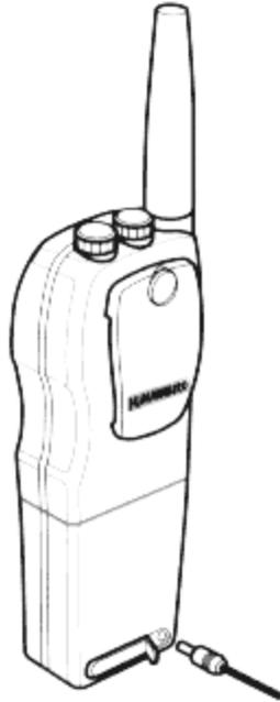
The battery drain is considerably greater when transmitting than receiving. A battery charge can be maintained for 8 hours or more (depending on ambient temperatures) when receiving only. Frequent transmitting, especially on High (5 Watt) output power will significantly increase the battery drain.
