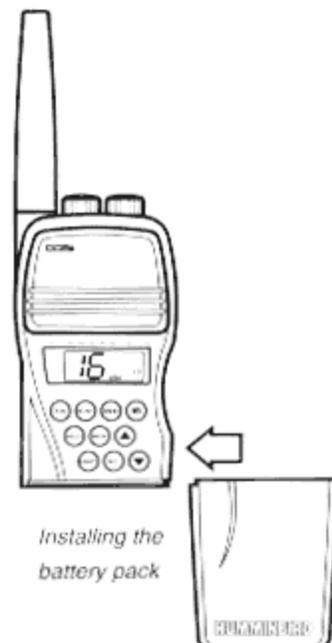
When the battery pack is off the DC5s unit, care should be used to prevent damage to the mating slide and electrical contacts on the top of the battery. Also the slide and contact area on the bottom of the unit will be vulnerable to damage if not protected. It is best to keep the battery pack installed even if the radio is being stored for extended periods.
