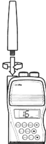
The antenna supplied with your DC5s is specifically tuned to optimize the radio's transmit power and the sensitivity of the receiver. To install, ensure the threaded base and the recessed threads on the unit are free from debris, and screw the antenna into the base. Finger tighten only.
