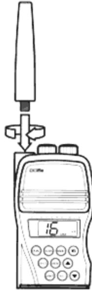
If you choose to use the belt clip included with your DC5s, simply fasten it to the mounting point using the attached screw. A flat head screwdriver or a small coin can be used. Do not over tighten the screw or use a fastener other than the one supplied.
