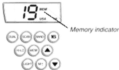
By pressing MEM, the Memory function is selected and the MEM enunciator will be continuously displayed. When in the MEM function, only channels stored to Memory will be accessible. The Up and Down arrow keys can be used to select any channel stored to memory. SCAN can be used to scan only the Memory channels.
