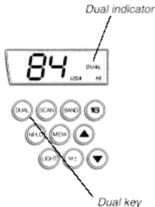
Select any channel on either USA or INT bands. Press DUAL. The DC5s will monitor your selected channel and channel 16 simultaneously. If a transmission is heard on either channel, that channel will continue to be selected until no further transmission is received, then dual watch will be re-engaged.
