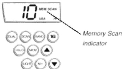
To delete a channel from Memory, select the Memory function and ensure the MEM annunciator is displayed. Use the Up or Down arrow button to select the channel to be deleted, and press M+/. The channel is now deleted from memory.
