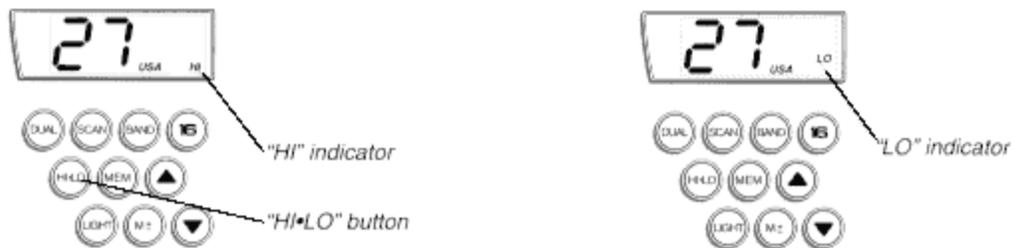
Selection of certain channels will cause the DC5s to automatically select the LO power output. This feature is required by the FCC.
