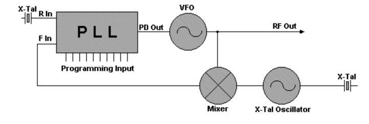
The output frequency can be changed by changing the mixing-xtal or add a new mixing-xtal to the oscillator.
