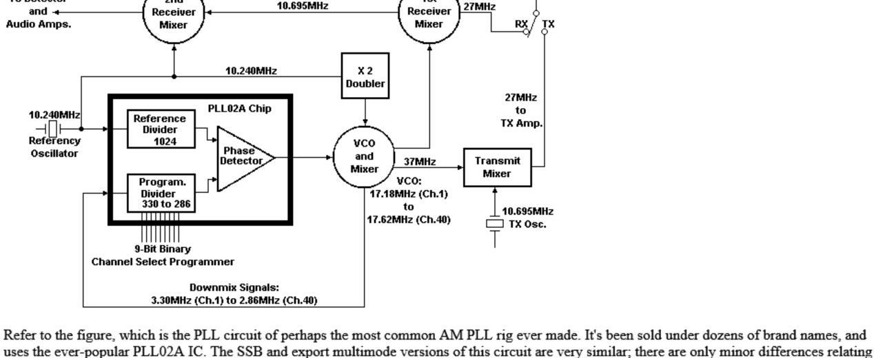
MHz. This particular example is actually the second generation of the PLL02A AM circuit; the original PLL circuit used a total of 3 crystals. The key to synthesizing all of the required frequencies lies in the Programmable Divider. That's the only PLL section that you can control from the outside world by means of the Channel Selector. Which is where it all starts.
